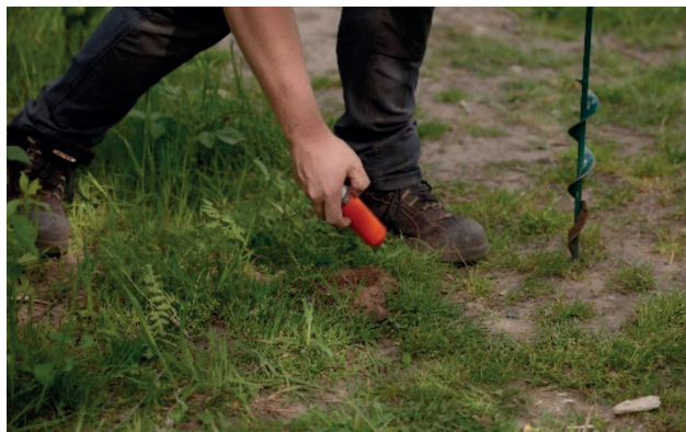
Figure 5 Stryde Node being deployed.
