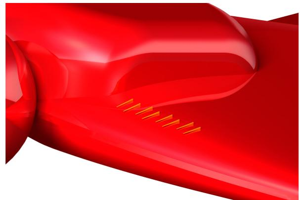
Figure 11.14: CATIA model of Vortex Generators, an overview (left) and a close-up (right)
