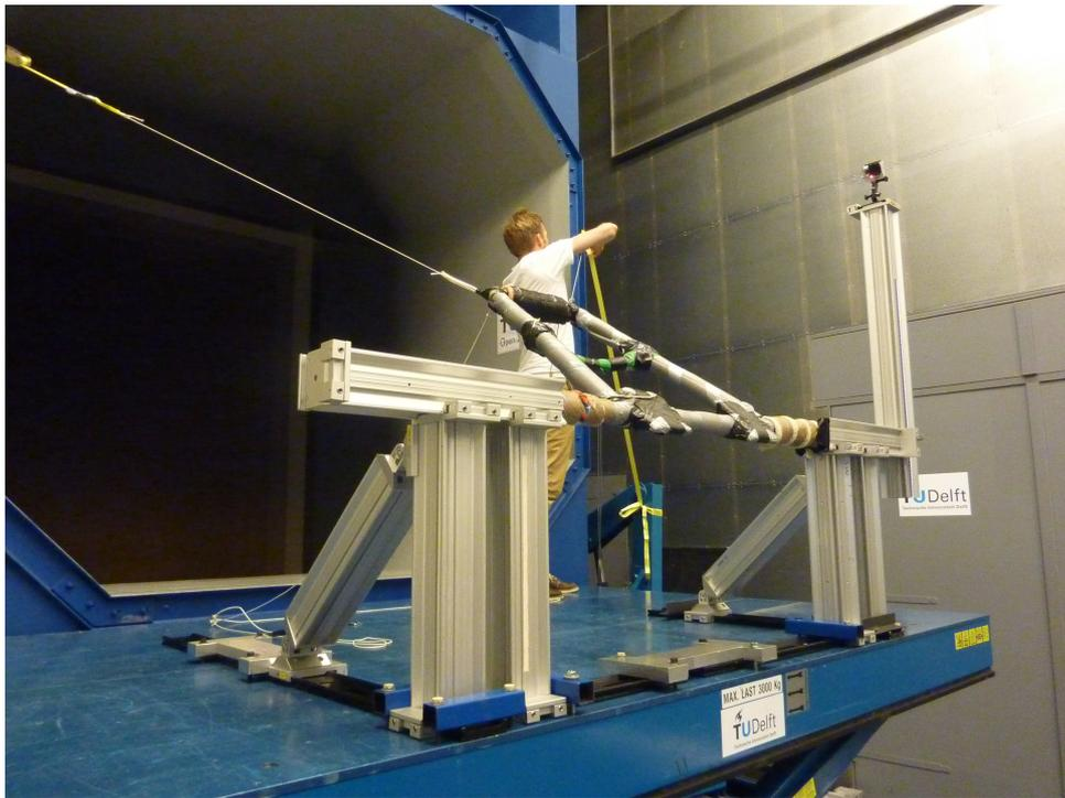
Figure 5.1: The structure used during the wind tunnel testing
