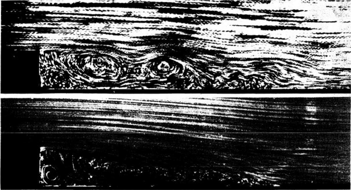
Figure 11.9: Aluminum-powder pictures of streamlines over a step. Exposure time 0.5(upper) and 5 seconds (lower) [51]
