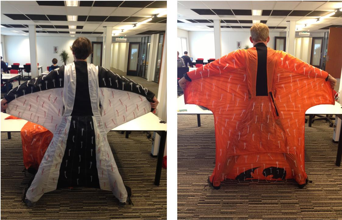
Figure 5.2: The wingsuit with tufts
