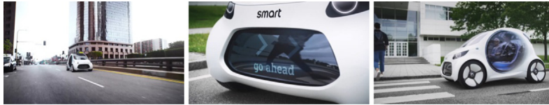
Car moves on road; '11th street' on the bumper, the car stops in front of zebra crossing; 'go ahead' and '>' sign appears on the bumper, and headlights turn into animated eyes; the pedestrian crosses (Daimler, 2017)
