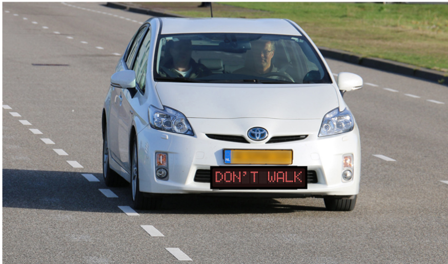
Fig. 5. eHMI concept 'DON'T WALK' in red letters overlaid over the photo. The person in the driver seat provided written consent for the publication of this photo. (For interpretation of the references to color in this figure legend, the reader is referred to the web version of this article.)
