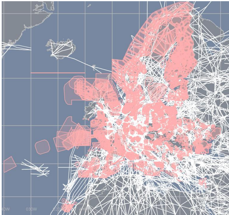
Figure 2.7: Special Use Airspace over Europe. Generated by Collaboration Human Machine Interface, CHMI
