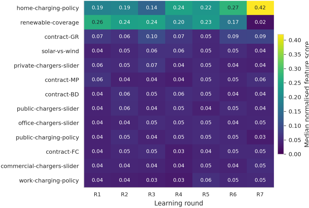
Figure F.2: Median normalised Extra Trees feature scores for log-transformed congestion loss across successive learning rounds, with both V2G model chains combined. The corresponding out-of-bag R^2 values averaged approximately 0.72.
