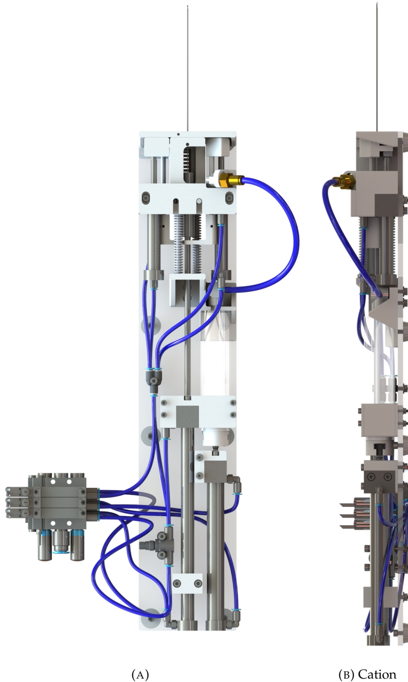
FIGURE G.5: Top (A) and front (B) view of the proof of principle prototype in Solid-Works. Figure shows both stylet and cannula in reloaded position.
