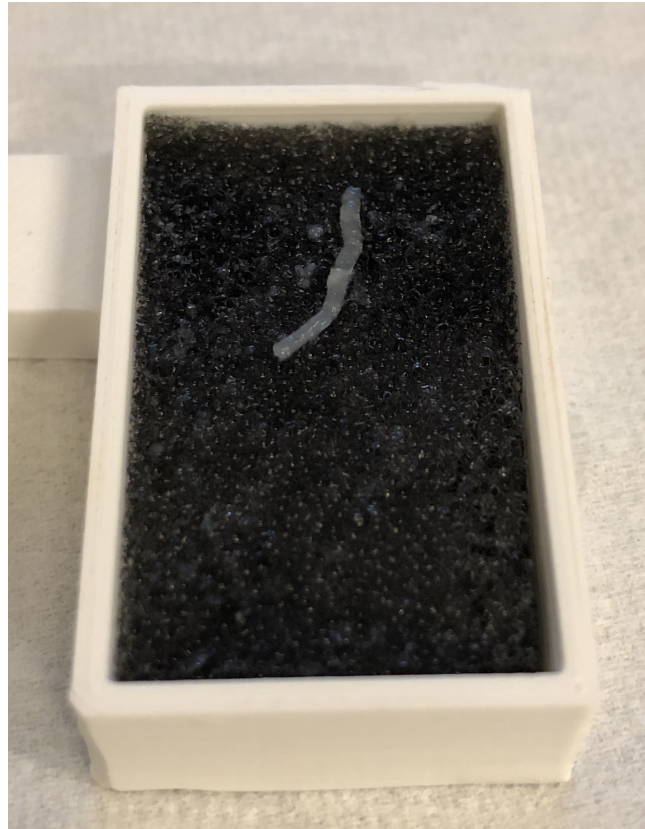
FIGURE 15.5: This figure illustrates a sample that was properly removed by flushing and deposited correctly in the container.
