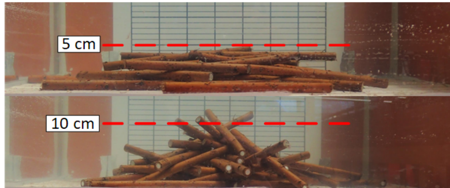
Figure 5.9: Difference in stacking behaviour (Top) Horizontally dropped (Bottom) Vertically dropped.
