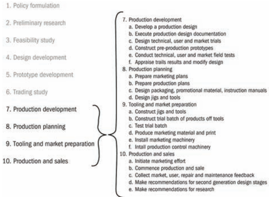
Figure 2.6 The ten steps of product innovation and the activities of the last four stages. (based on Archer 1971)
