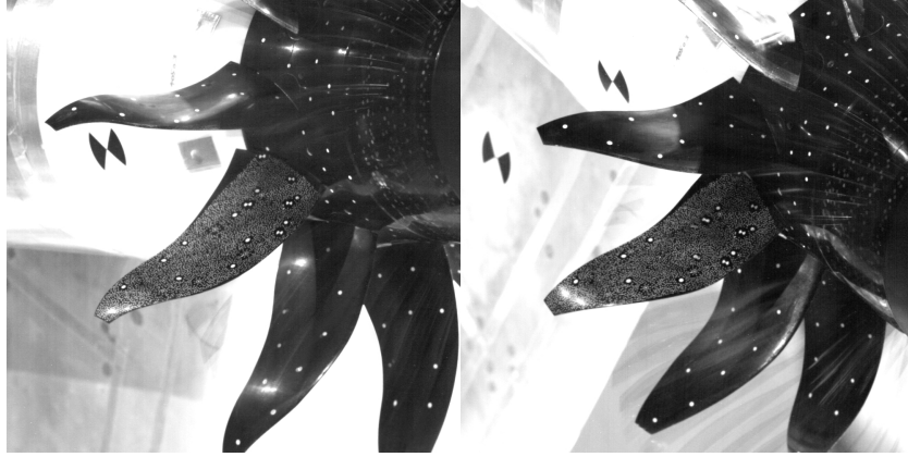
Figure A.5: Glare issue on the reference images - (Digitally distorted).
