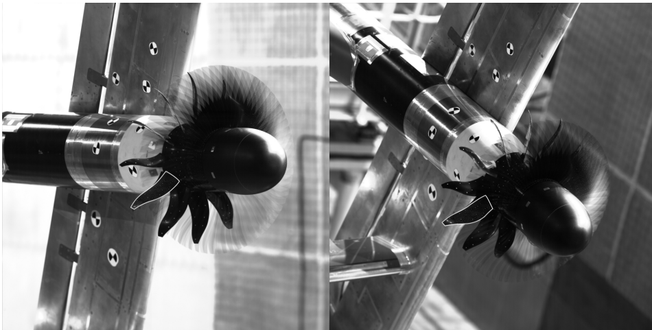
Figure A.4: Merged stator reference images, with the complete surface visible. - (Digitally distorted images)
