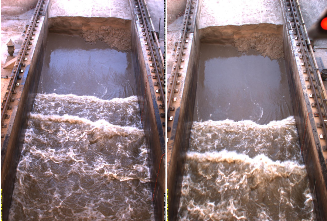
Figure 3.4 Snapshots of the same moment in test T06E by camera C1 (left) and camera C2 (right). In the upper part of the images the dune face is visible. The led light captured in the image of camera C2 is used to synchronise video images with in-situ pressure and velocity measurements.
