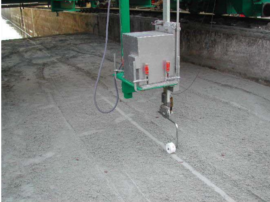
Photo A.1 Amphibious profile follower, here positioned on top of the dune
