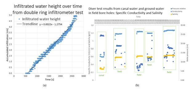
Fig. I.3: Data obtained from field measurements in selected field in Fidel Castro drainage system near Xai-Xai city, Mozambique. (a) Double ring infiltrometer test infiltration rate. (b) CTD-diver data in canal water and different bore holes in field.
