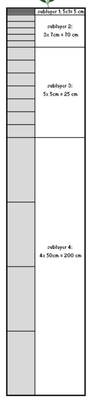
Fig. 2.11: Applied soil layering in SWAP
