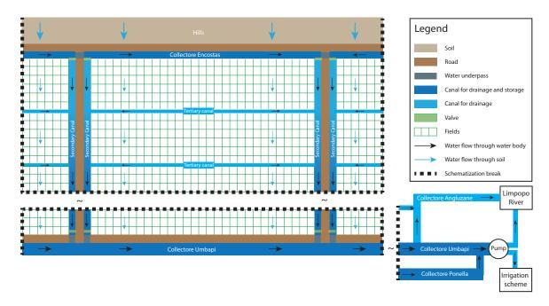
Fig. 3.11: Schematization of the agricultural system in the Fidel Castro irrigation/drainage block near Xai-Xai Mozambique, within the area of the Regadio do Baixo Limpopo (RBL). The observed field is located in this area.
