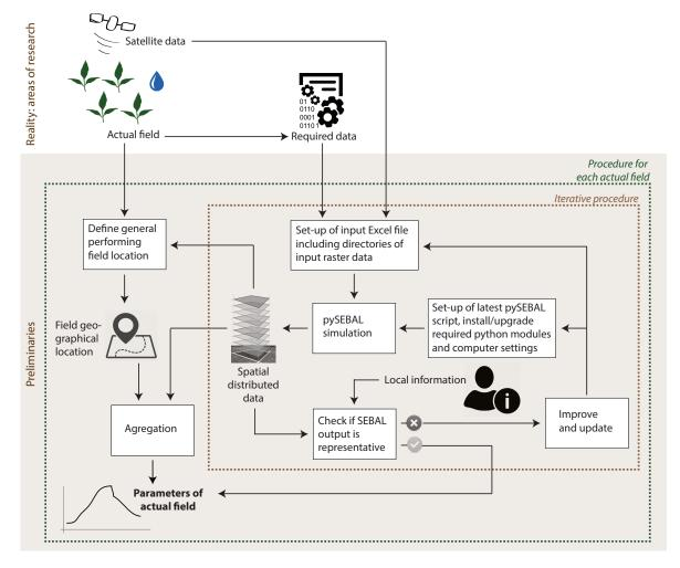
Fig. 2.6: Application of SEBAL to obtain parameters of actual field
