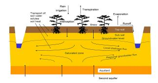
Fig. 2.8: The SWAP model domain and transport processes described by Kroes et al. (2009)
