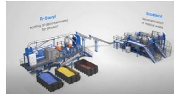
Figure X: Ecosteryl decontamination and R-Steryl sorting installations and recovered streams (R-steryl : Decontaminated Medical Waste Sorting Center, 2023).
