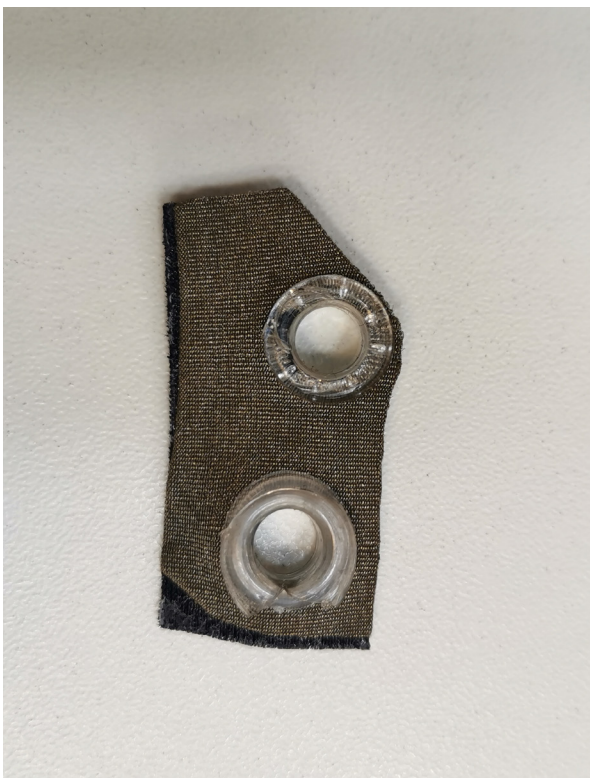
Figure 131: Successful eyelet ring(top) and failed eyelet ring(bottom)
