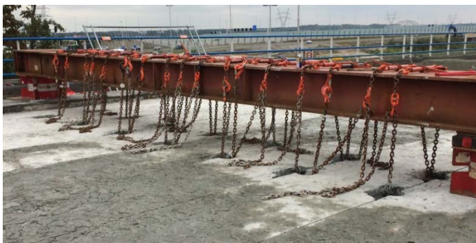
Figure 6 Safety system for single beam tests (steel chains), top side (left), bottom side (right).
