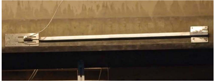
Figure 7 Vertical LVDT at support (left), horizontal LVDT at bottom flange beam (right)
