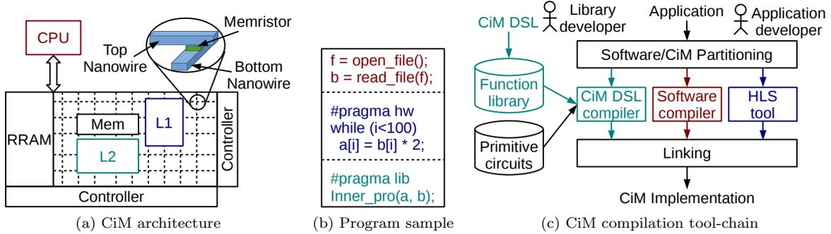
Figure 1: CiM architecture and compilation tool-chain.
