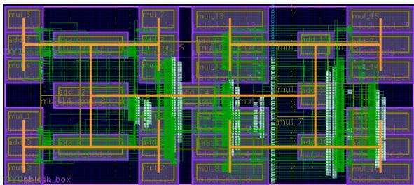
Figure 8: FPGA floorplanning for inner product.
