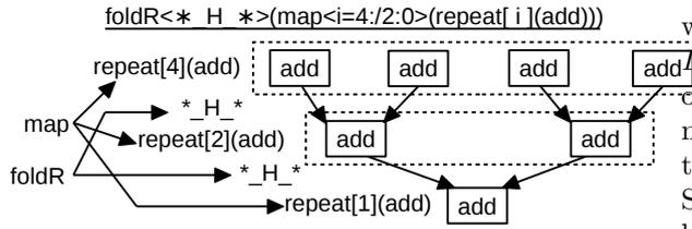
Figure 4: Expression and data-flow graph of an adder tree.
