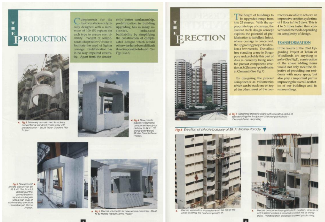
(Fig. 26) Trade journal article showing the process of fabricating and grafting new pre-cast volumes onto existing housing blocks. Housing and Development Board, 'Public Housing Upgrading: New Frontiers in Prefab Applications', Structech News 10 (December 1993): 1-4. Collection of the National Library Board of Singapore.
