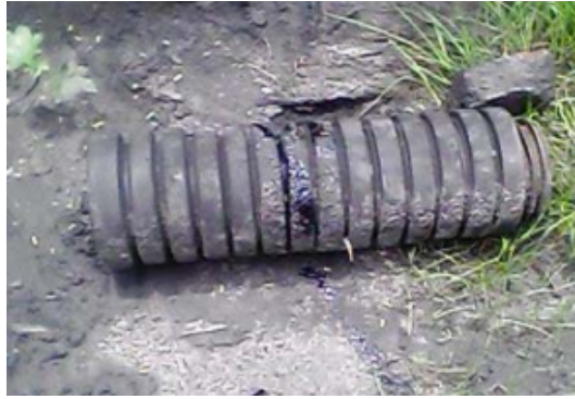
Figure 2.4: Idler roller wear [4]
