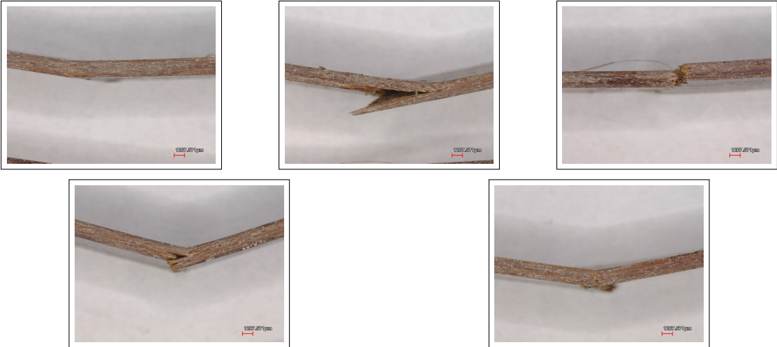
Figure D.9: 2-NaBF showing minimal delamination with mainly tensile failure of outer fibres
