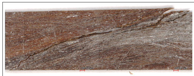
(b) 8-NaBF specimen showing debonding-based failure with failure along the fibre
