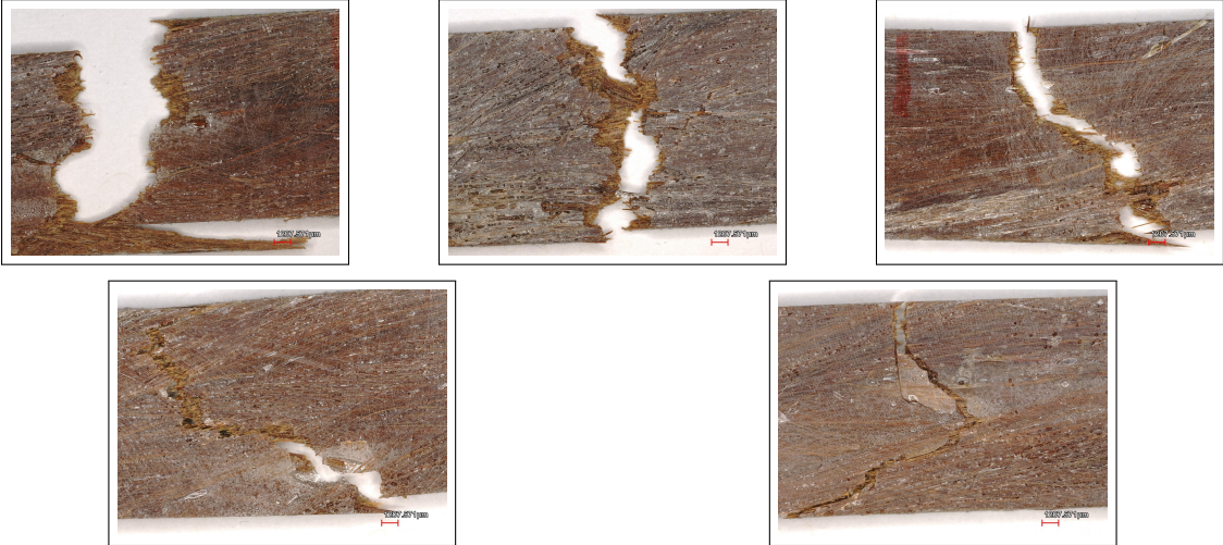
Figure D.3: 5-NaBF laminate showing varied failure modes and high void content
