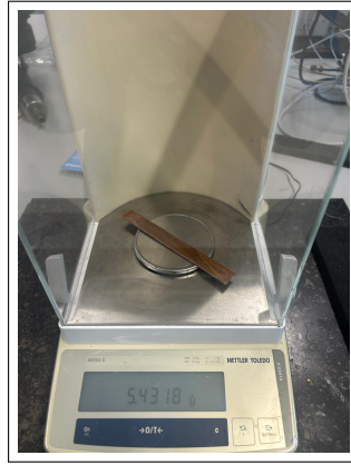
Figure 4.15: Specimen weighing using the Mettler Toledo scale
