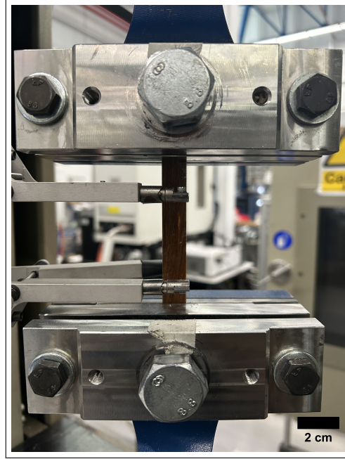
Figure 4.18: Tensile testing setup on the 20kN UTM with extensometer for accurate measurement of displacement
