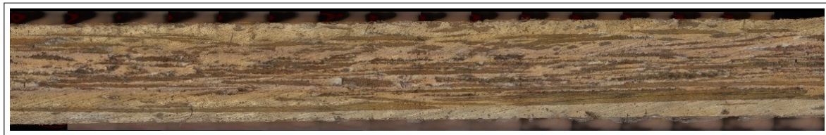
(a) Untreated showing good fibre-matrix distribution, fibre alignment and low void content
