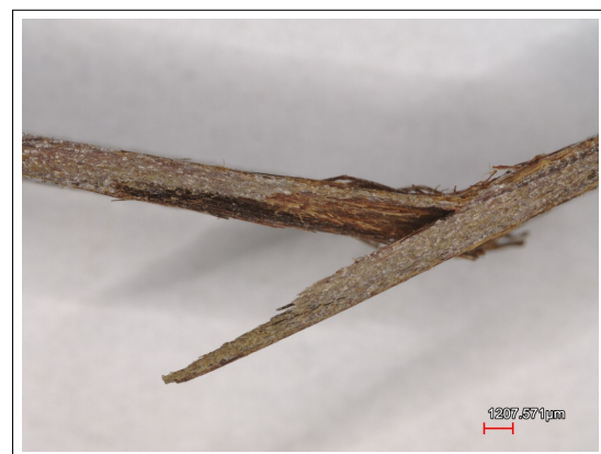
(b) 8-NaBF specimen showed fibre rupture and debonding
