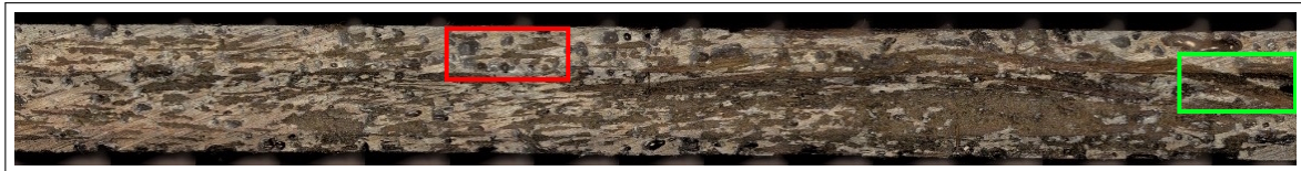
(d) 8-NaBF shows highest void content, dry regions and fibre degradation throughout the specimen
