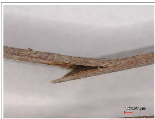
(a) 2-NaBF specimen showing fibre-matrix debonding in the middle
