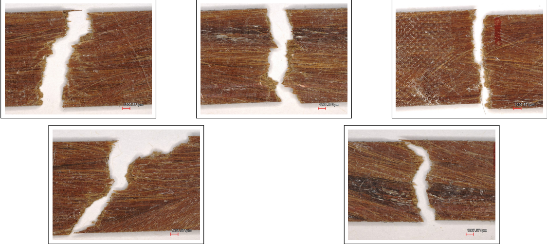
Figure D.2: 2-NaBF laminate showing mainly fibre failure with void present
