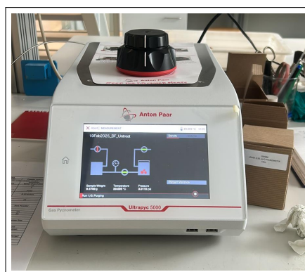
Figure 4.3: Anton Paar Ultrapyc 5000 with the digital display indicating the current status of the experiment. The specimen chamber can be seen here with the black cover on top.
