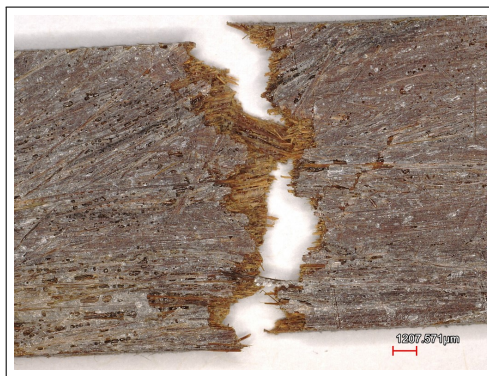
(a) 5-NaBF specimen showing signs of poor impregnation and fibre-matrix debonding
