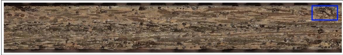
(c) 5-NaBF with higher and more regular void regions with fibre misalignment and dry spots
