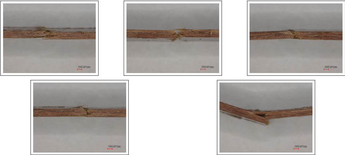
Figure D.13: 5-SiBF showing primarily brittle failures with minimal fibre-matrix debonding
