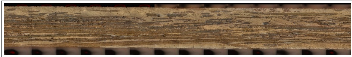
(e) 2-SiBF with much improved laminate quality despite some non-uniformity in fibre-matrix distribution
