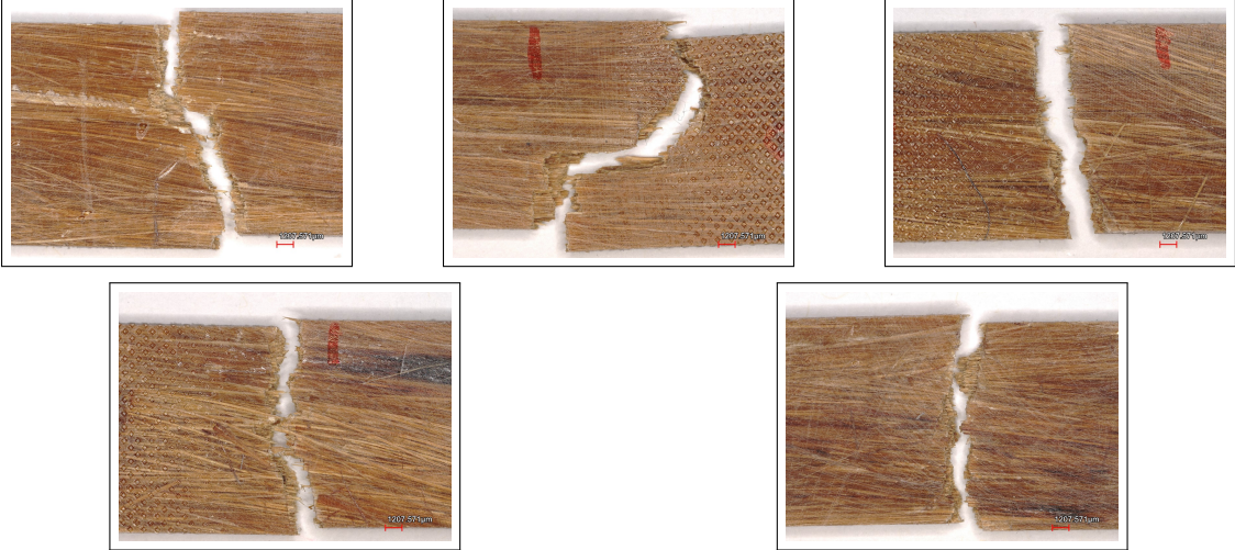
Figure D.5: 2-SiBF laminate mainly showed fibre failure with some debonding visible
