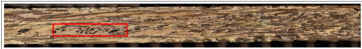
(g) 8-SiBF shows a single region with high void content, which could be due to fibre misalignment issues
