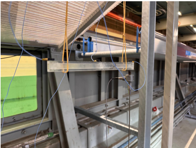
Figure A.48: Specimen testing set-up example, Clear resin.
