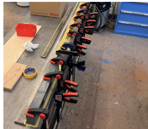
Figure 17: Indicative beam assembly and curing procedure.
