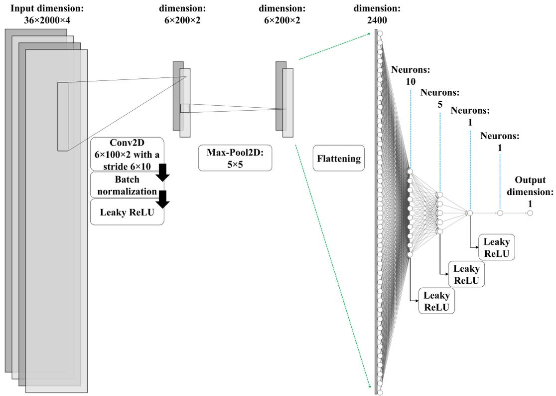
Figure 2. The architecture of the proposed CNN model.
