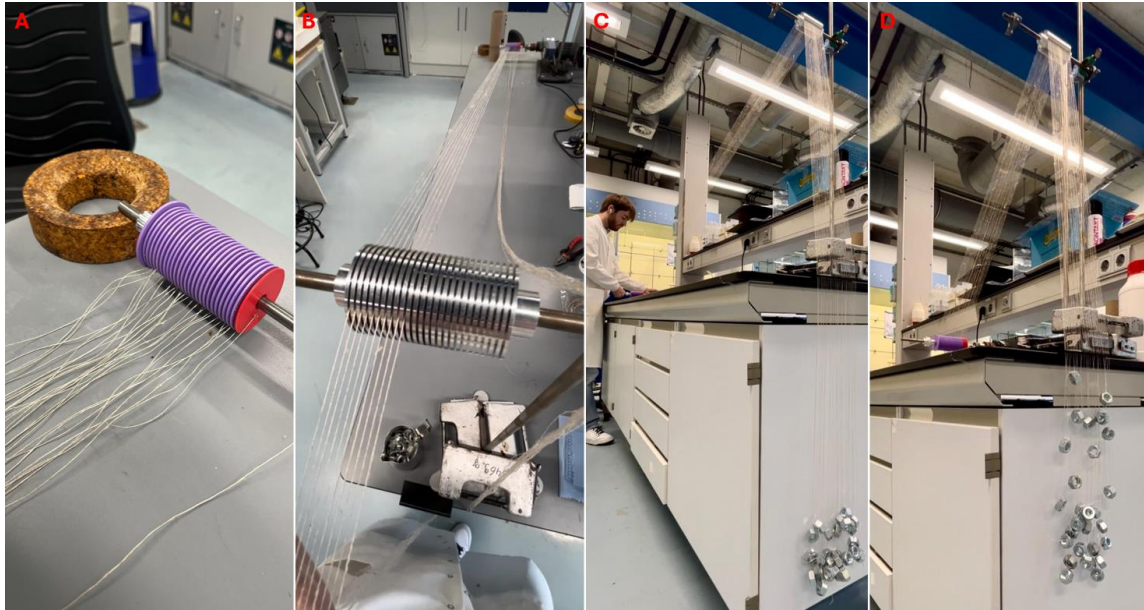
Figure 21: (a) Flax yarns tied on the feeder slots. (b) Process of passing the yarns through the splitter and the guiding holes. (c) Start of the winding process. (d) End of the winding process, the feeder has been moved closer to the splitter in order to wind the yarns.
