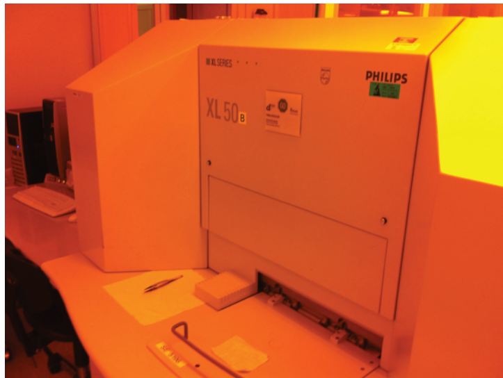
Figure 3.5: Philips XL-50 SEM system in PVMD/DIMES clean room.
