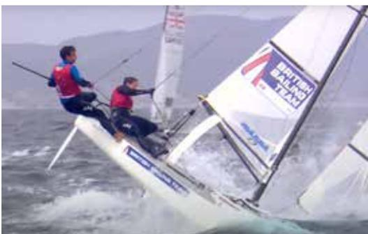
Fig.2.16 A pitchpole. One of the hulls slips below the waterline and the whole boat flips. A dangerous situation. A crewmembers are often thrown overboard in these situations.
