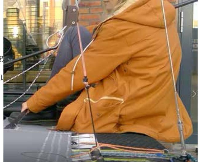
*Fig.3.24 Lifting the hiking strap with the hand to get the foot in.*
