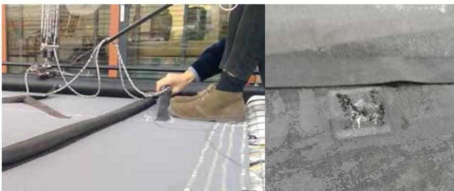
*Fig.5.6 Left: participant of the dry test lifting up a hicking strap. Right: ripped off and often restitched hicking strap*
