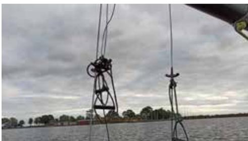
*Fig.3.19 helmsman trapeze wire is made defunct*
