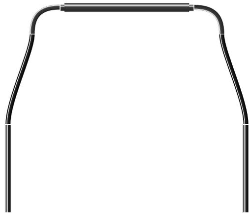
Fig.5.2 Two detachable S shaped tubes are added to place the crossbar forward of the main sheet. The joystick can be removed with the already existing clip system.
