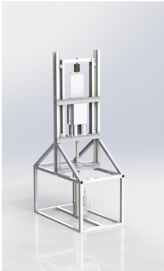
FIGURE A.1: Render of the Vertical Adhesion Test Setup
