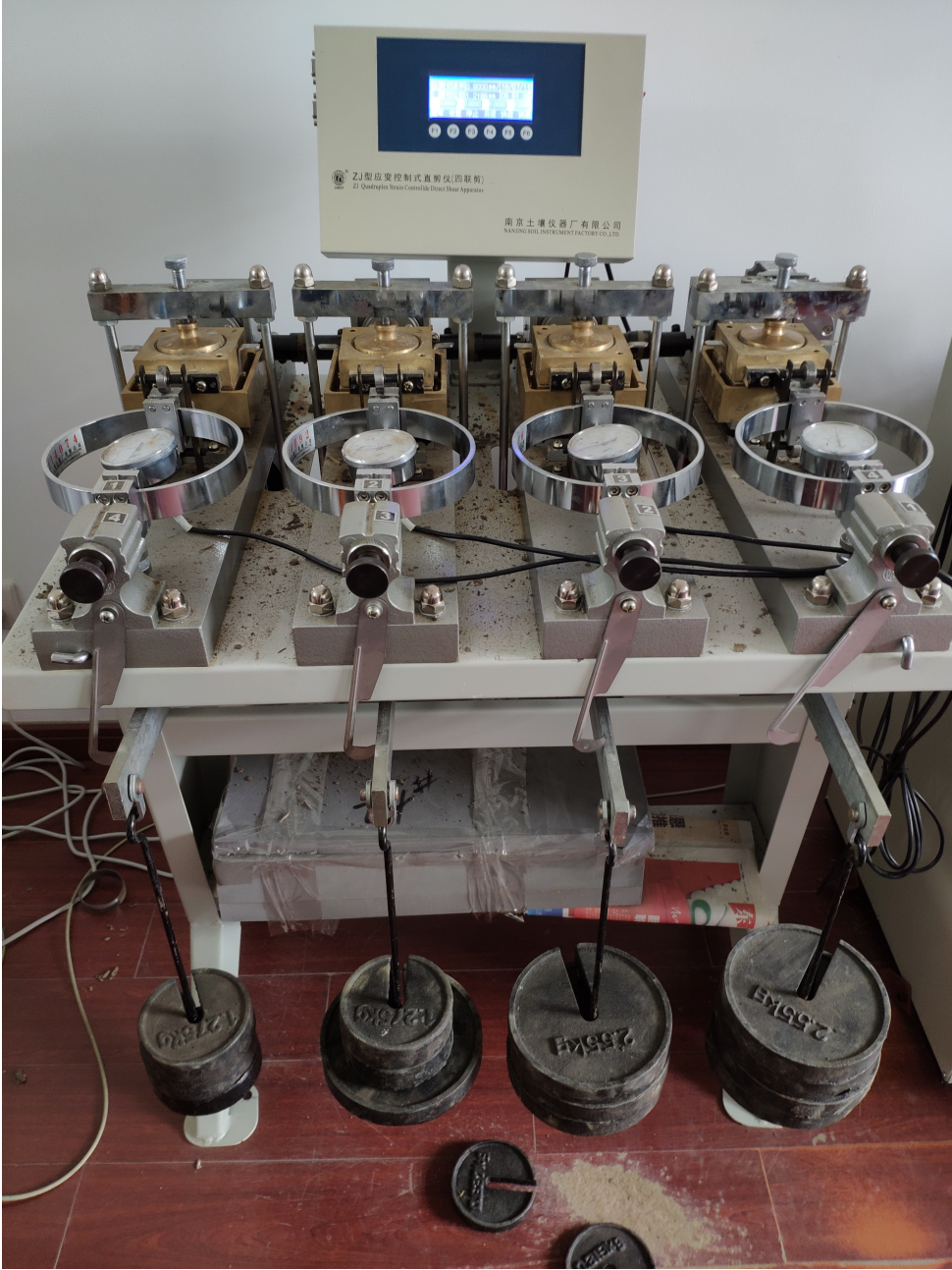
FIGURE A.3: The direct shear apparatus used to measure the undrained shear strength
