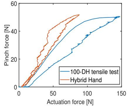
Figure 20: Amplification pinch force test for the parameters:  $f_{amp} = 1.5$ ,  $k_p = 0.5$ , and an allowable error of the motor position of 2 degrees. The limit of the maximal amplification of pinch force has been set to 20 N.
