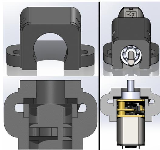
Figure 9: Left: Designed motor bracket with inner blocks. Right: Assembly of the motor bracket and the motor. The round shape at the front of the bracket allows the axial bearing to also refrain the motor shaft from bending due to radial forces.
