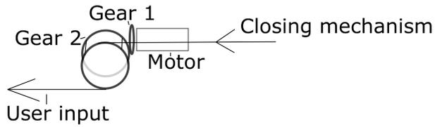
Figure D.2: Concept 2: Actuator drives a pulley (with gear transmission) which is directly connected to a pulley of the user input.
