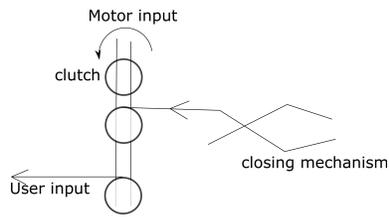
Figure D.1: Concept 1: Actuator input coupled with a one-way clutch to the user axis. This allows the user to overrule the system in terms of closing the hand. For opening the hand the actuator should be used.
