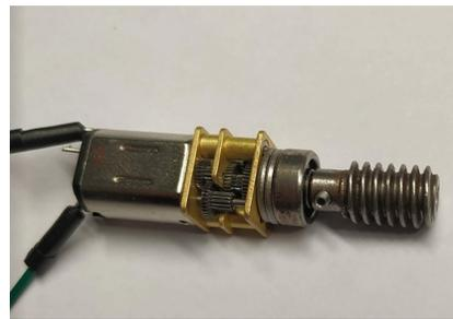
Figure E.5: Due to the axial load one of the gears is pushed against the housing, resulting in high friction.
