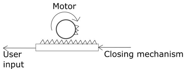
Figure D.4: Concept 4: An element with a linear gear is moving along a rotation point of the motor when the user actuates the cable. By actuating the motor the pinch force can be amplified. The teeth of the motor pulley grip into the element of the user input.
