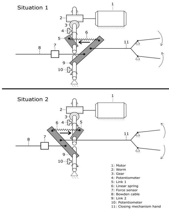
Figure 8: A systematic overview of the final solution. In Situation 1 the motor helps the user to close the hand and amplify the actuation forces of the user; the spring-force on the base crank of the user is directed to the left. In Situation 2 the spring force on the base crank of the user is directed to the right, thus closing the hand.
