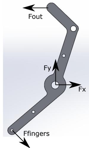
Figure A.6: Free body diagram of the finger link
