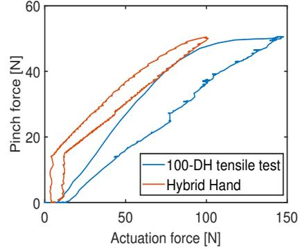
Figure 19: Amplification pinch force test for the parameters:  $f_{amp} = 1$ ,  $k_p = 0.9$ , and an allowable error of the motor position of 2 degrees.
