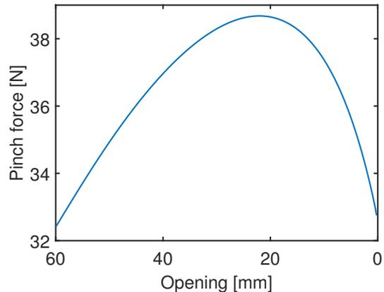
Figure 4: With an input force of 100 N the output pinch force has been plotted against the opening of the hand. At 60 mm opening the hand is completely open and at 0 mm the hand is completely closed.
