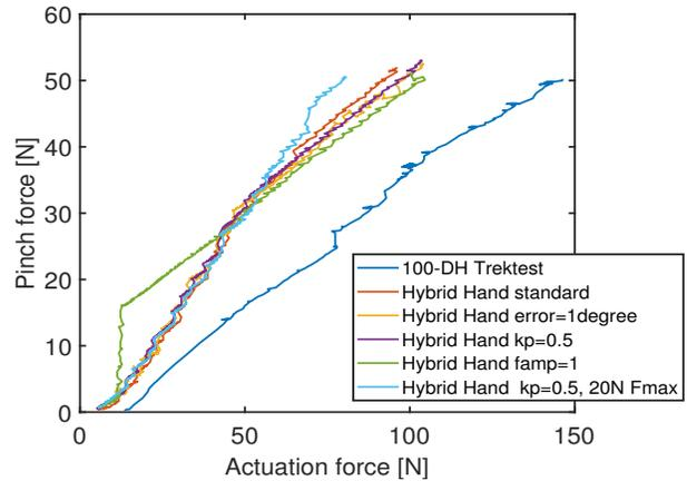
Figure 22: All of the pinch force amplification tests plotted in one figure. For readability only the closing of the hand has been plotted. The complete cycles can be found in Section 7. Evaluation tests.
