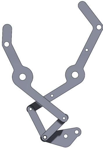
Figure A.1: Closing mechanism with all of the linkages
