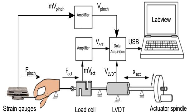
Figure 5: Test set-up used for testing the transmission ratio of the 100-Dollar Hand. Adapted from [21].
