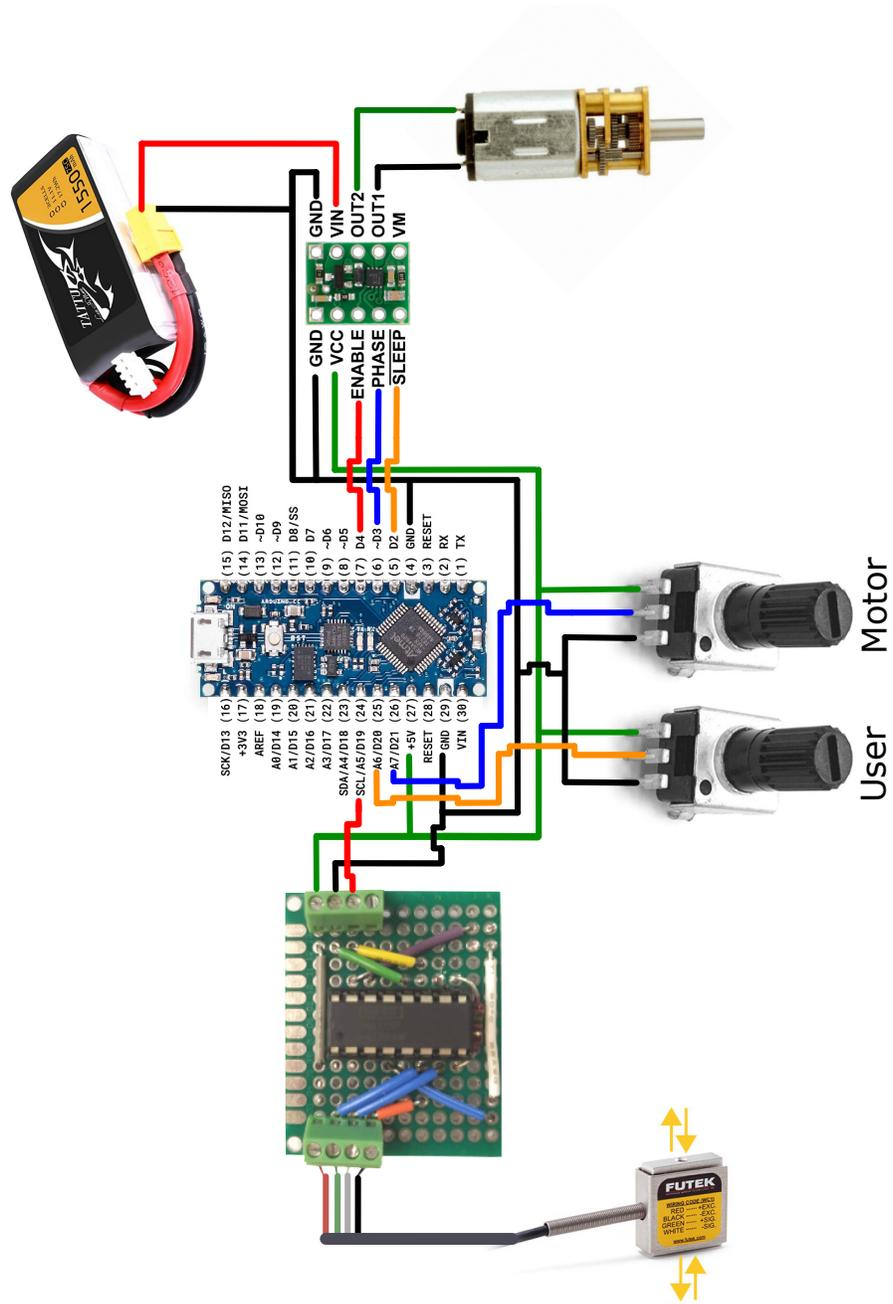
Figure H.3: Electric scheme of the Hybrid Hand with all the components and sensors included.
