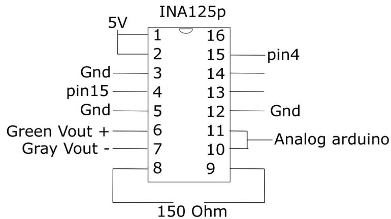
Figure H.2: Connection scheme of the INA125p amplifier
