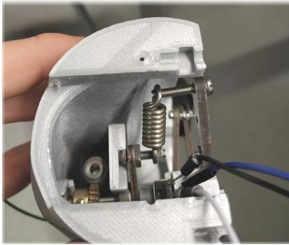
Figure E.1: Spring has been aligned so that the horizontal forces are minimal.
