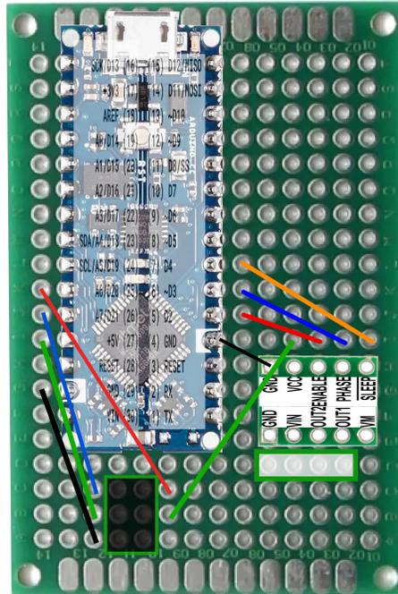
Figure H.1: PCB of the Arduino and motor driver.
