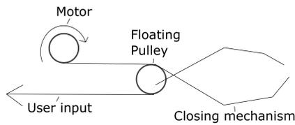
Figure D.5: Concept 5: The user actuates a floating pulley which can move horizontally. To amplify the pinch force the motor drives the pulley from the other end of the rope. By changing the closing mechanism a rotation pulley could also be viable.
