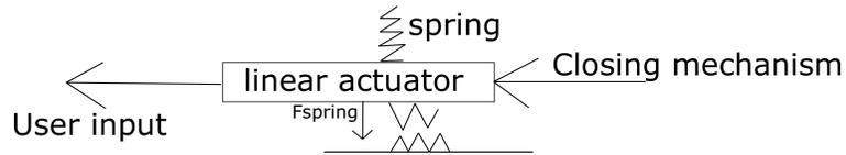
Figure D.3: Concept 3: Linear actuator which grips into teeth of a gear when spring force presses the actuator down. When gripped to the shell the linear actuator can amplify the pinch force.
