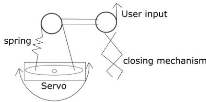
Figure D.6: Concept 6: Series elastic actuator, a servo actuator is attached with a spring and a cable to 2 sides of a pulley. The pulley is connected to the user pulley and input with a shaft (possibly a clutch). By controlling the servo's position the spring will be tensioned and adds forces to the user input.
