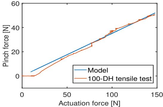
Figure 7: The scaled closing mechanism compared to the tensile test of the 100-Dollar Hand.
