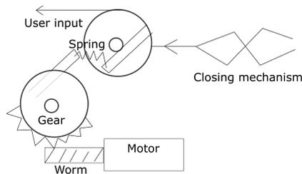
Figure D.8: Concept 8: Final concept, by controlling the position of the gear on the motor side, the spring can be tensioned to amplify the forces of the user to open or close the hand. When using a worm gear as transmission, the motor can stop when the desired position is reached.
