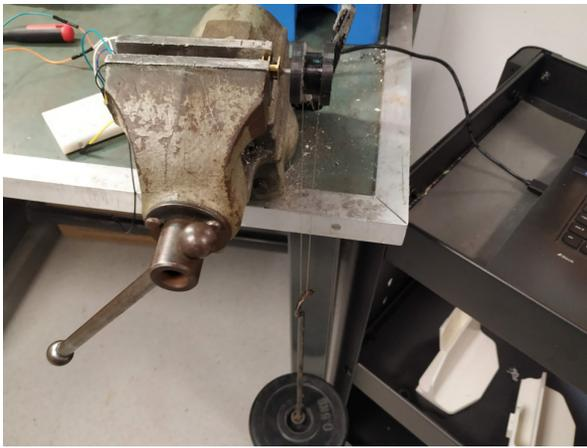
Figure E.2: A pulley has been attached to the motor shaft. The weights are elevated on a 1 cm radius
