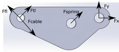
Figure A.3: Free body diagram of the base link
