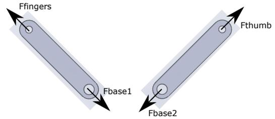
Figure A.4: Free body diagrams of the 'floating' thumb and finger link
