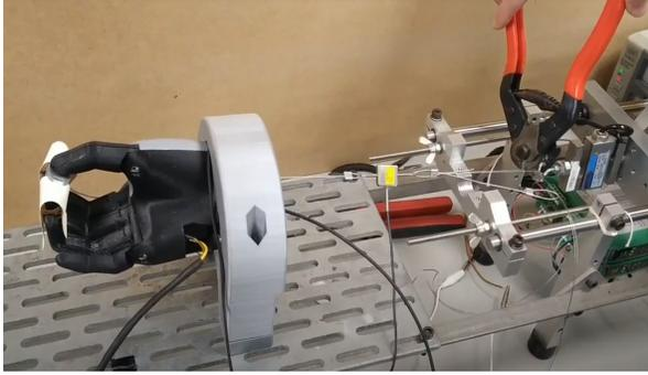
Figure 21: Test set-up of the quick release test. With a pinch force of 30 N, the cable is cut using pliers.
