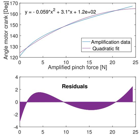
Figure 14: Example of a quadratic fit for the angle of the user crank where the hand opening is 10 mm. The residuals of the fit can be seen in the second plot. An accuracy of around 2 N can be seen.
