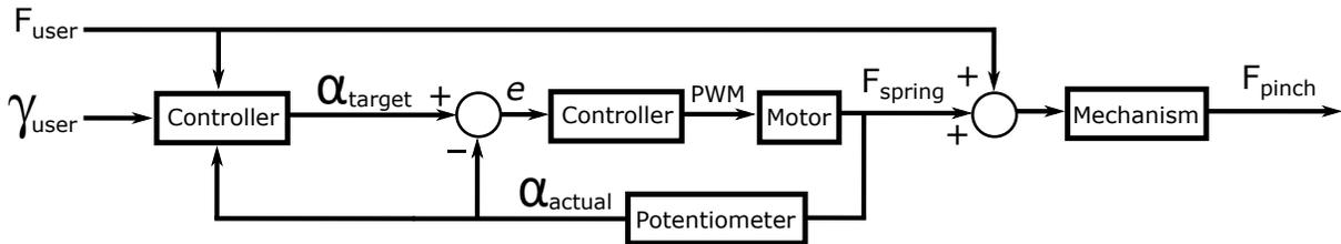
Figure 10: Control block scheme. The controller calculates the target location for the motor from the angle of the user base crank ( $\gamma_{user}$ ), the user actuation force ( $F_{user}$ ) and the actual position of the motor base crank ( $\alpha_{actual}$ ). The motor control loop is acting as a servo motor control loop. The output pinch force is a result of two forces acting on the user base crank: user actuation force and spring force.
