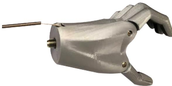
Figure 2: The 100-Dollar Hand with Bowden cable. At the base of the hand a screw can be seen, so that the hand can easily be mounted to a socket.
