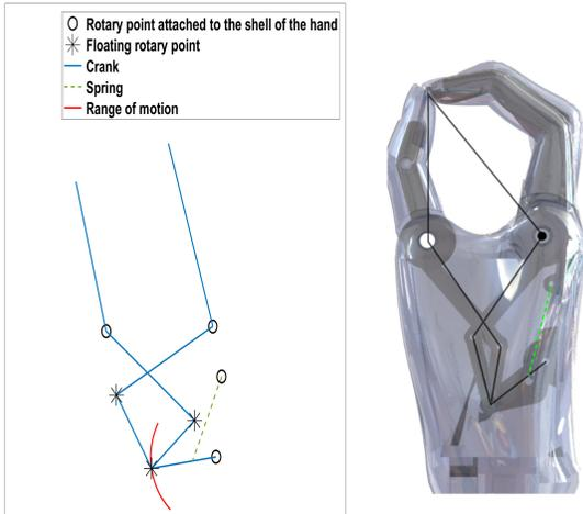
Figure 3: Analyses of the closing mechanism. Left: The mechanism of the simulation model plotted. Right: Solid-works version of the 100-Dollar Hand, lines have been added to clarify how the simulated version compares to the real model.
