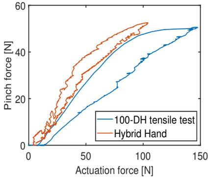
Figure 17: Amplification pinch force test for the parameters:  $f_{amp} = 1.5$ ,  $k_p = 0.9$ , and an allowable error of the motor position of 1 degree.
