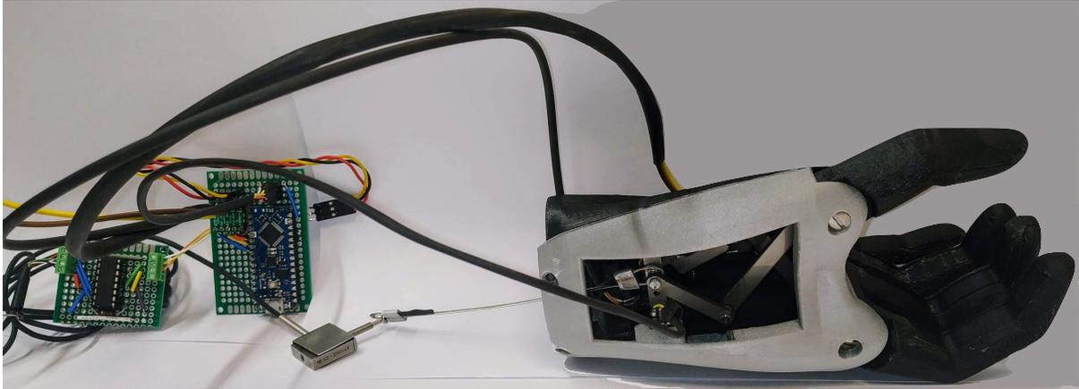
Figure 12: Complete system of the Hybrid Hand. Via a viewing hole in the outer shell the mechanism can be observed. Three cables come from the hand to the soldered PCBs, 1 for the motor and 2 for the potentiometers.
