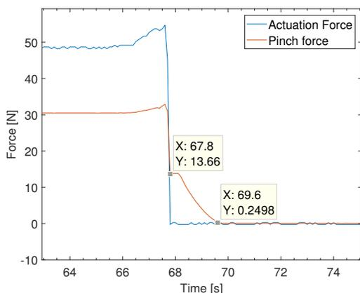
Figure 23: Results of the quick release test. With start conditions: motor amplification of 14 N and a total pinch force of 30 N.
