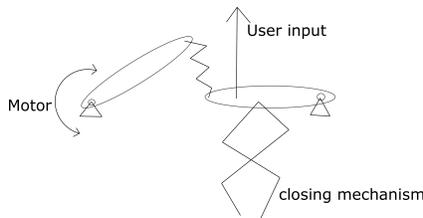
Figure D.7: Concept 7: Series elastic actuator, by changing the output torque of the motor the spring can be tensioned both ways. This allows for control of an added moment force for closing and opening the hand.
