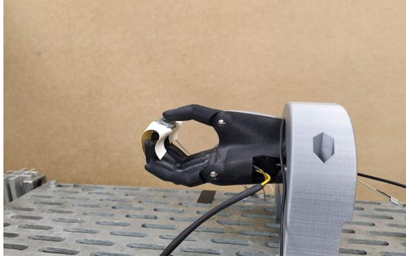
Figure 15: The prototype clamped to the test set-up, by increasing the angle of the motor crank the maximal pinch force can be tested.
