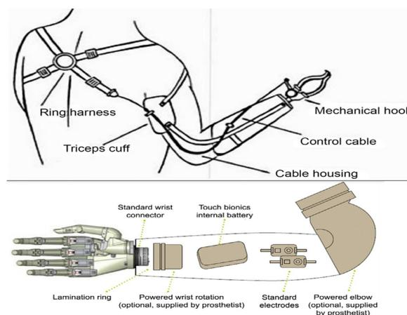
Figure 1: Types of active prostheses. Top: Working principle of the voluntary closing body-powered prosthesis. When the cable is pulled the hand closes. The user can pull the cable by extending his/her arm or by using their opposite shoulder [13]. Bottom: Example of a myo-electric prosthesis (i-Limb). The electrodes pick up a signal from the users muscles and translate this signal to opening and closing the hand[14].
