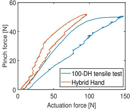
Figure 16: Amplification pinch force test for the parameters:  $f_{amp} = 1.5$ ,  $k_p = 0.9$ , and an allowable error of the motor position of 2 degrees.
