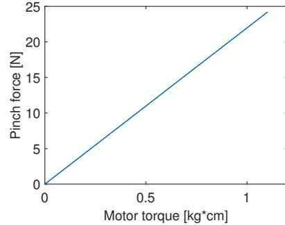
Figure 11: Motor torque plotted against the pinch force amplification, with a worm gear efficiency 0.9.
