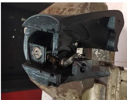
Figure E.3: A bearing has been added in the extension of the motor shaft, this prevents the worm from slipping on the gear
