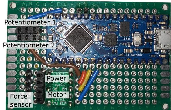
Figure 13: PCB with the motor driver and the Arduino. For each of the sensors a connection plug has been made. This way broken sensors can be replaced quickly.
