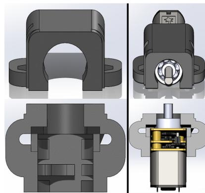
Figure E.6: Left: Designed motor bracket with inner blocks Right: Assembly of the motor bracket and the motor. The round shape at the front of the bracket allows the axial bearing to also refrain the motor shaft from bending due to radial forces.(Duplicate of Figure 9 for clarity reasons)
