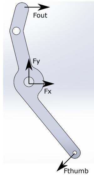
Figure A.5: Free body diagram of the thumb link
