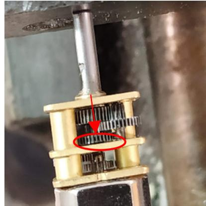
Figure E.4: Due to the axial load one of the gears is pushed against the housing, resulting in high friction.
