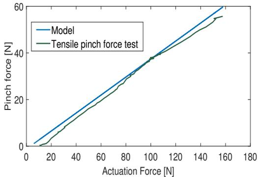
Figure 6: Tensile comparison of the model with the 100-Dollar Hand. The model slightly overestimates the pinch force for each actuation.
