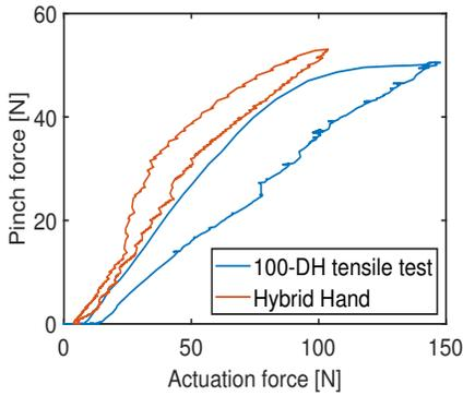
Figure 18: Amplification pinch force test for the parameters:  $f_{amp} = 1.5$ ,  $k_p = 0.5$ , and an allowable error of the motor position of 2 degrees.
