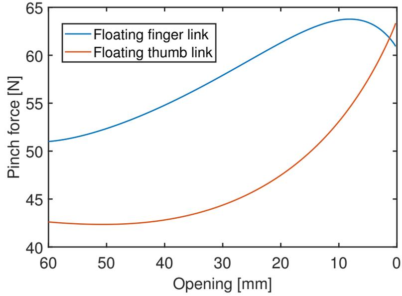
Figure B.1: Forces of the two floating links
