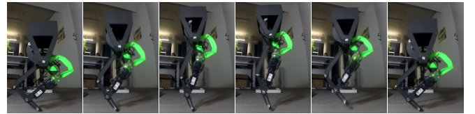
Fig. 7: A series of stills taken from a video of the jumping experiment, showing one jump from lower apex to consecutive lower apex.
