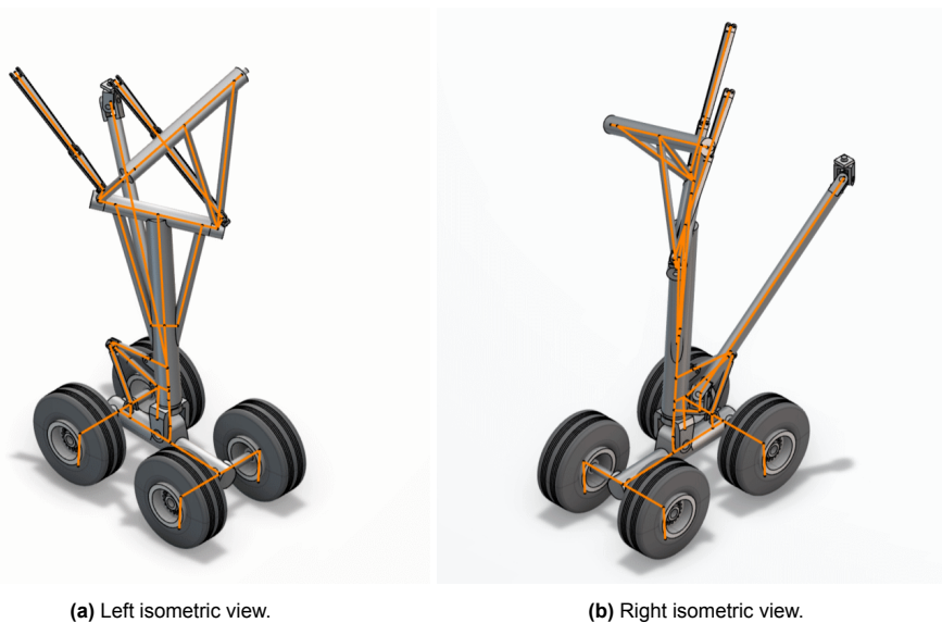
Figure 5.28: FV-1000 reverse stowage concept (C5) right main landing gear 3D model and refined stick model in orange.
