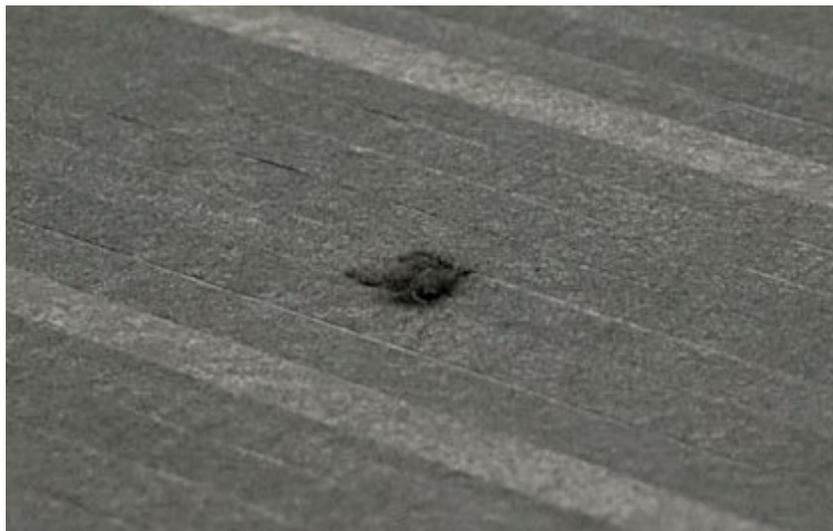
Figure 2.5: Fuzzball that contaminates the laminate formed by abrasion of fibre material [18] (Courtesy of Netherlands Aerospace Centre (NLR))
