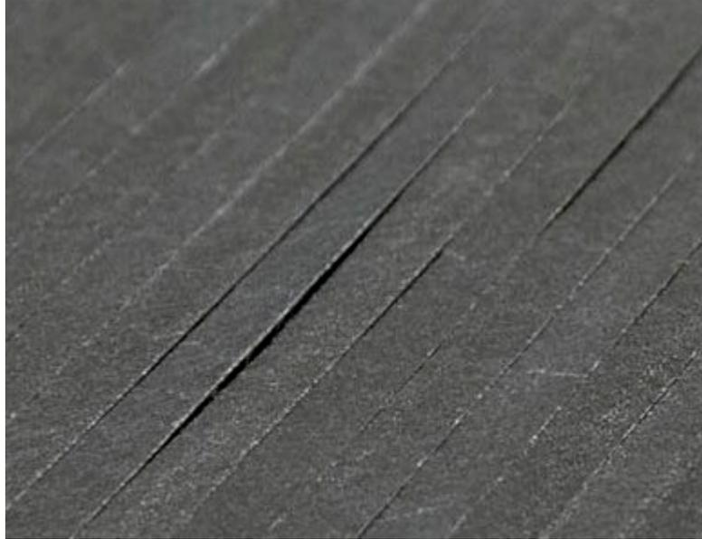
Figure 2.4: Tow upfolding due to lack of tackiness [18] (Courtesy of Netherlands Aerospace Centre (NLR))
