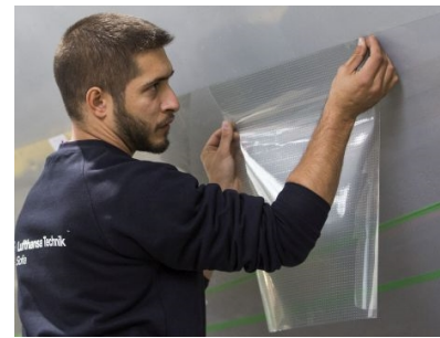
Figure 15.4: Riblet technology installation
