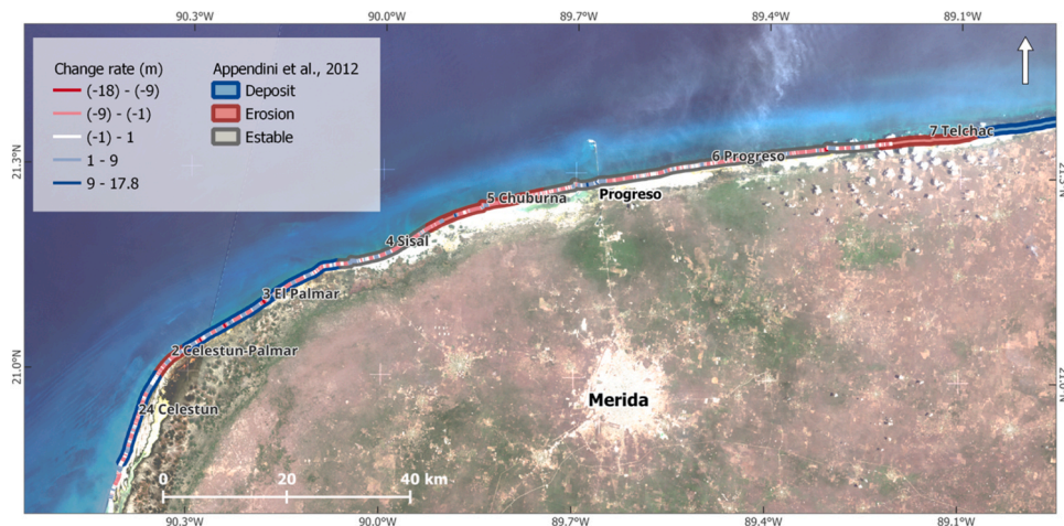
Fig. 8. Shoreline evolution as predicted by potential sediment transport gradients in Appendini et al. (2012) (outlines) and estimated from Sentinel-2 images (cross-shore transects).
