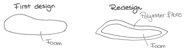
Figure 73 - Addition of polyester fibre
