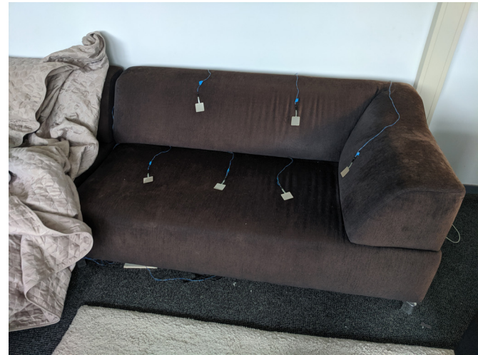
Figure 7 - FSR placement on the couch
