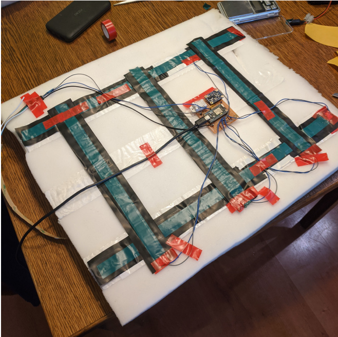
Figure 81 - Placement of BNO055
