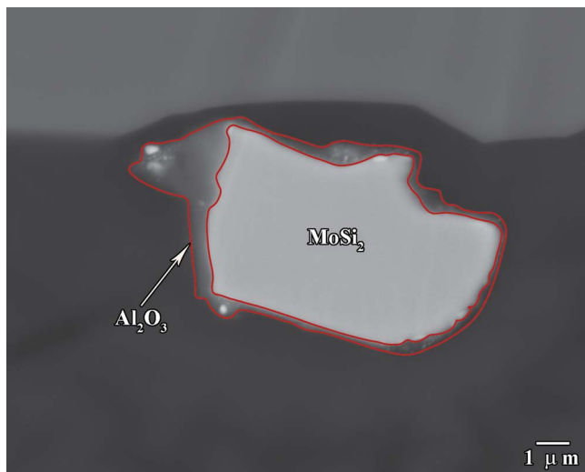
Fig. 6. Cross-section image of encapsulated MoSi 2 particle with a shell of Al 2 O 3 after annealing at 1200 °C for 1 h in Ar.
