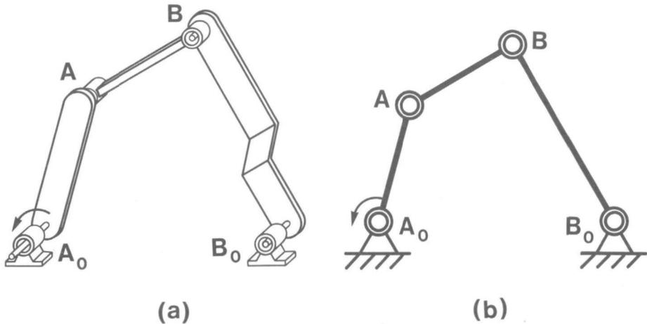
Fig. 23 Planar mechanism (a) and coplanar model (b).
