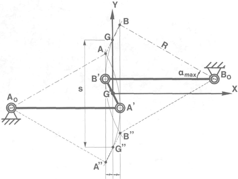
Fig. 15 Watt's straight-line mechanism.
