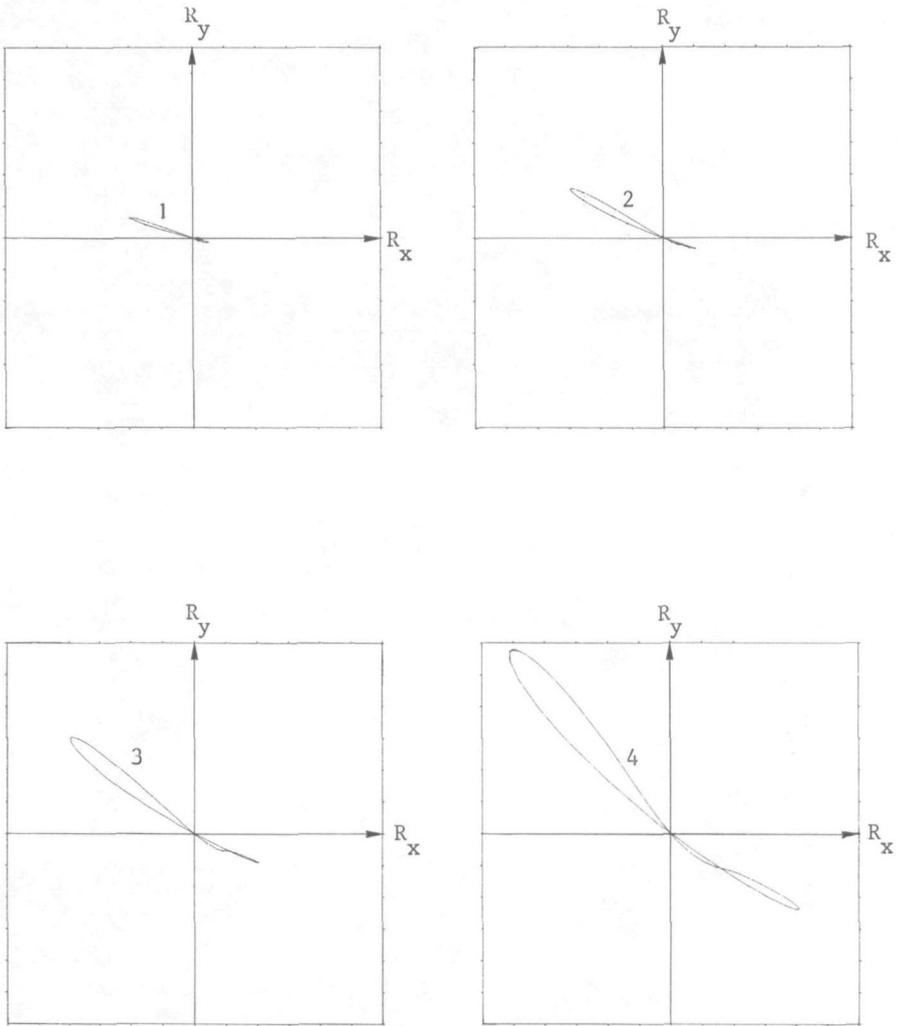
Fig. 33 Polar plot of crankshaft bearing force.
