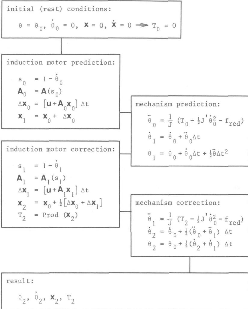
Fig. 19 Integration of induction motor-mechanism system.
