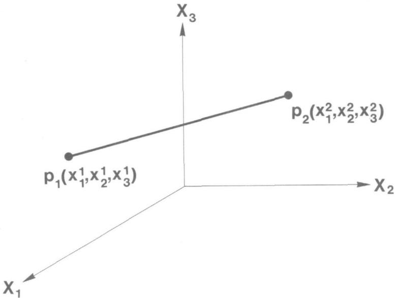
Fig. 6 The spatial truss element.
