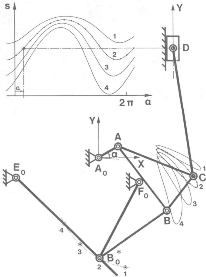
Fig. 29 Pouliot engine, kinematical results.
