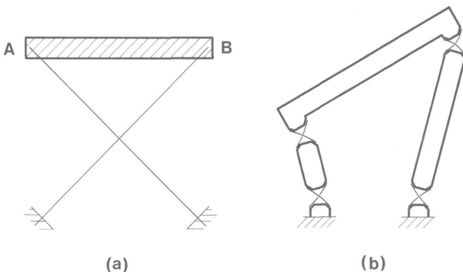
Fig. 1 Cross spring pivot and four-bar with cross spring pivots.
