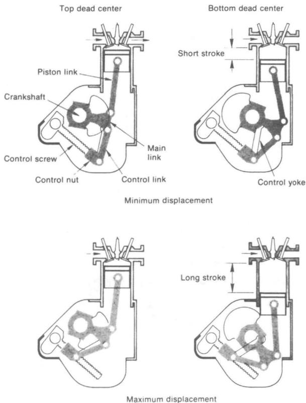
Fig. 27 The Pouliot engine [22].
