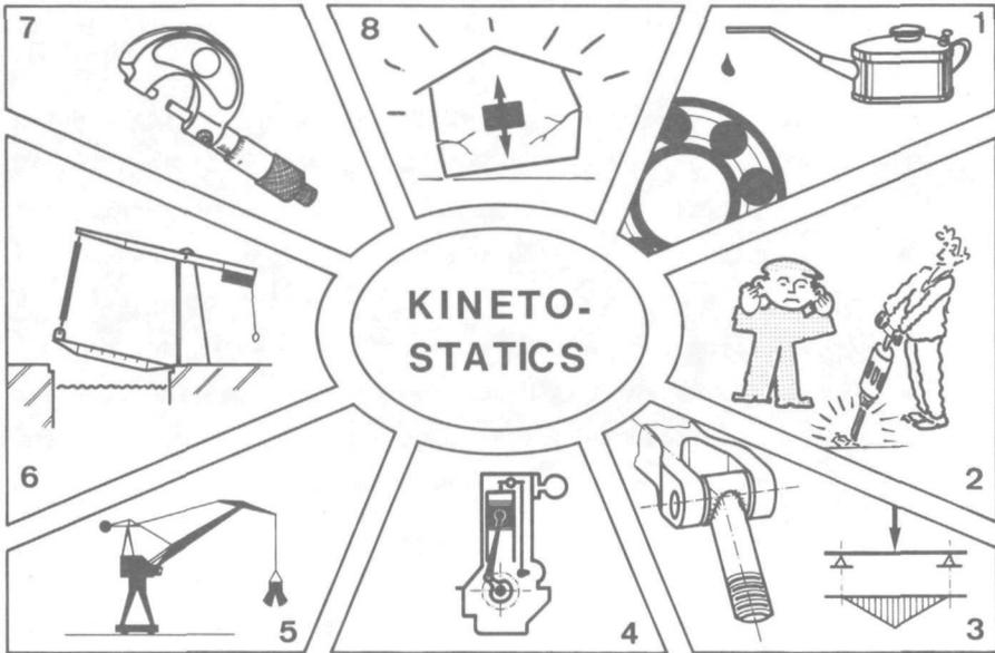
Fig. 25 Keyrole of kinetostatic analysis: bearing forces for the design (3), lifetime and service (1) of the connections, reaction forces for vibration nuisance (8), static and dynamic loads for balancing (6) and fatigue load (4,5), deflections for position accuracy (7).
