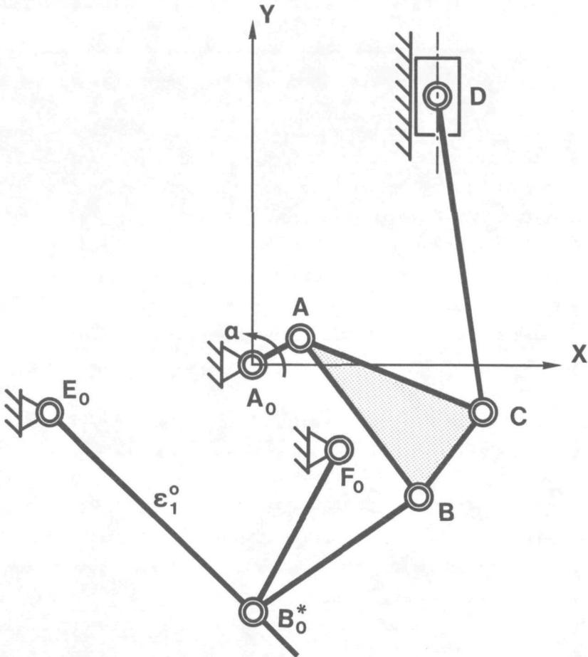
Fig. 28 Principle design of the Pouliot-engine.
