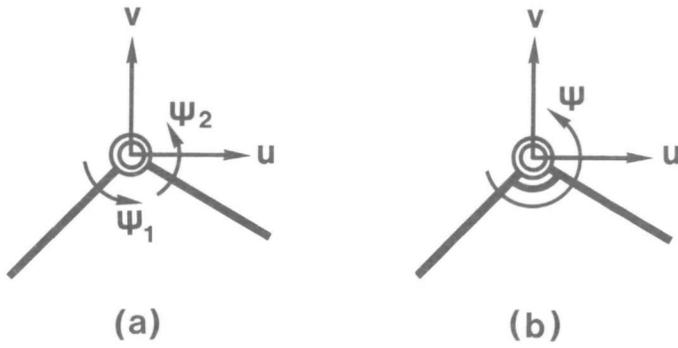
Fig. 9 Pin joint (a) and rigid connection (b).
