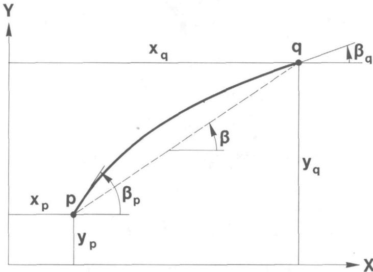
Fig. 4 The beam element: coordinates.
