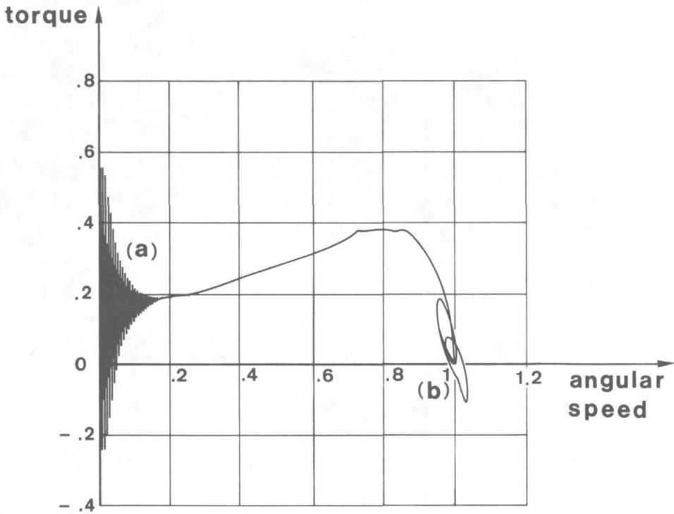
Fig. 20 Starting behaviour (a) and steady state solution (b).
