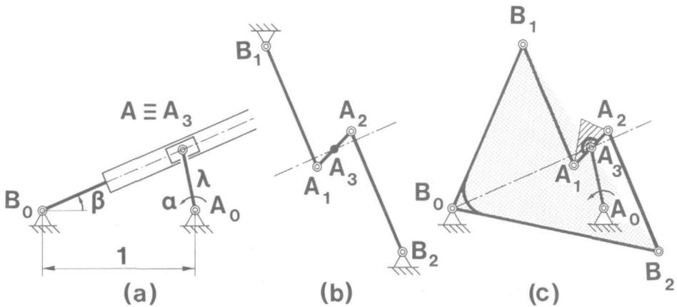
Fig. 14 Slider-crank (a), Watt's (b) and replacement mechanism (c).
