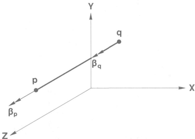
Fig. 5 The out of plane torsion element.
