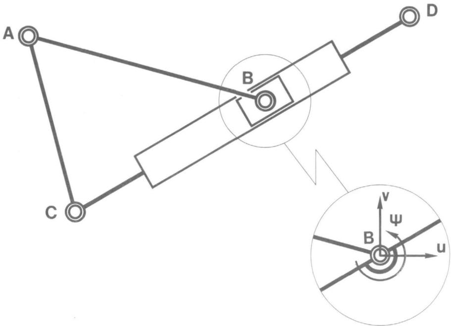
Fig. 10 Slide connection.
