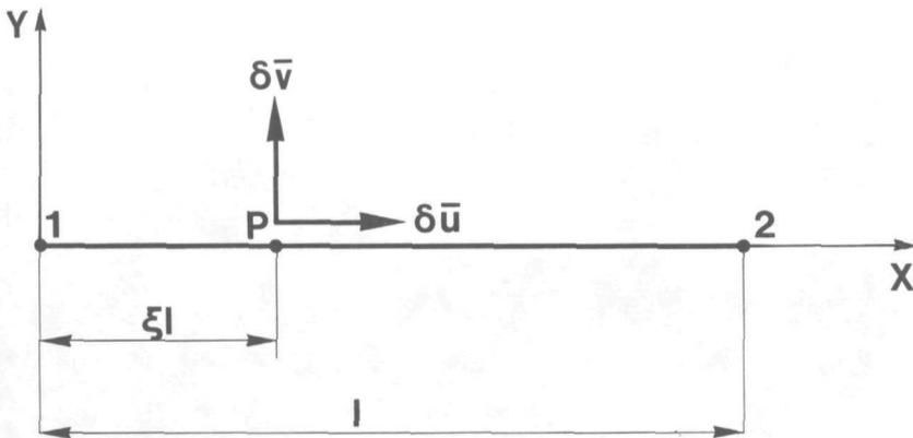
Fig. 18 Beam element in local coordinate system.
