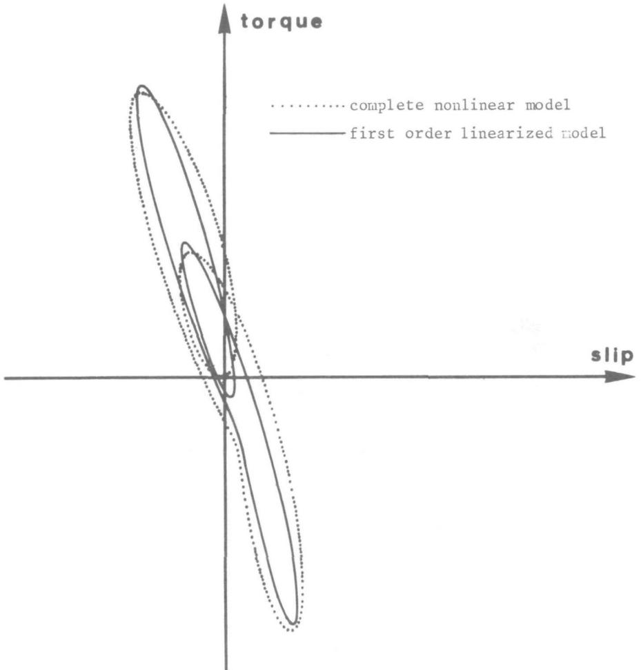
Fig. 21 Steady state slip torque diagram.
