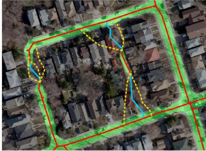
Figure 2.3: Connection hypotheses generated by the A^* search during the post-processing step in DeepRoadMapper. Retrieved from Mattyus et al. [49]
