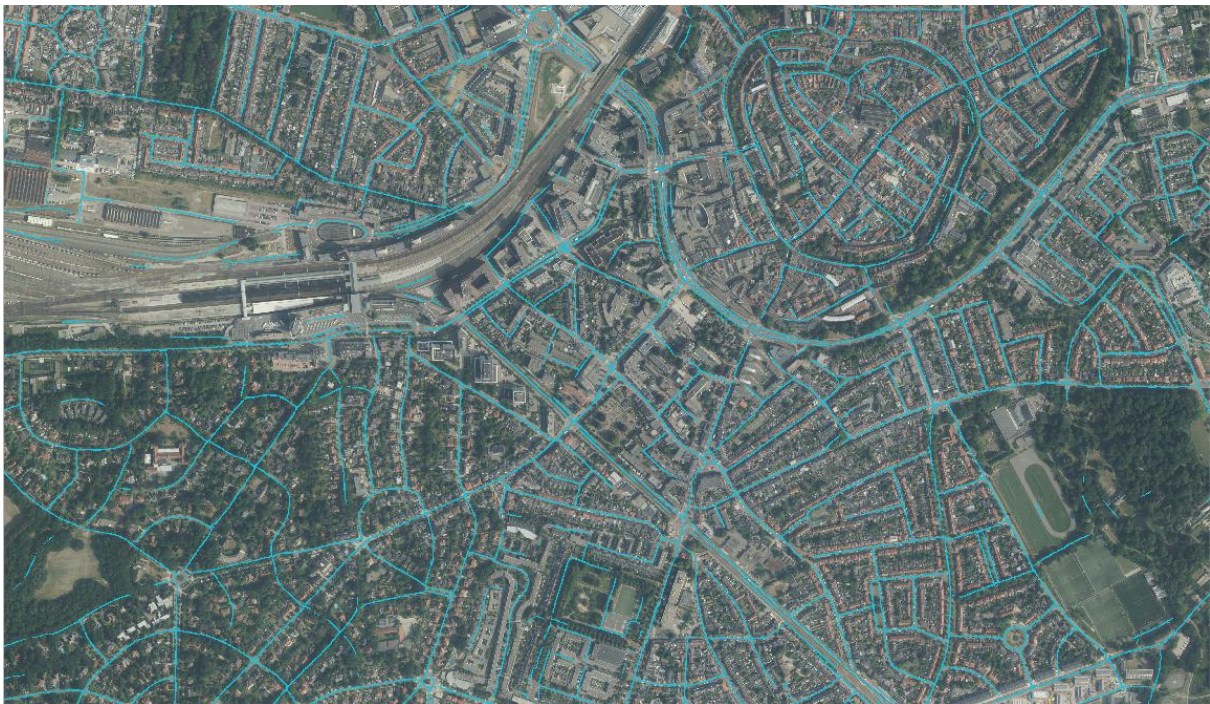
Figure 1.4: Example of Road Detection with Semantic Segmentation over a region in the Netherlands
