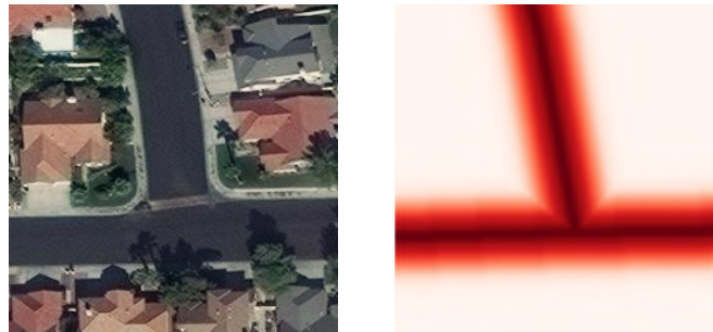
Figure 3.10: Gaussian Road Mask Learning task. From Left to Right: satellite image, corresponding ground truth mask
