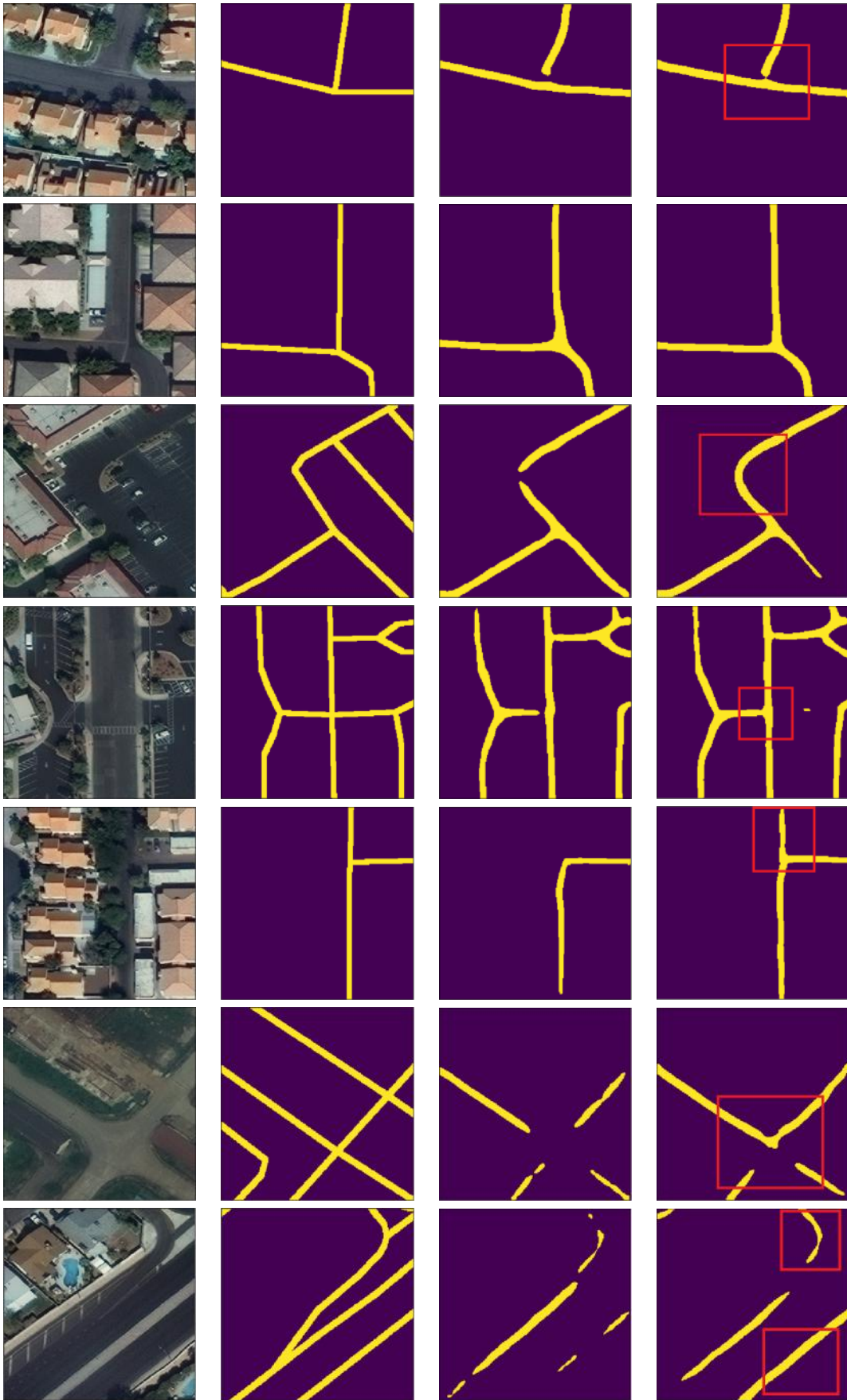
Figure 4.8: Visual inspection of the proposed model's performance. From left to right: satellite image, ground truth mask, single-task Road Detection Prediction, Multi-Task Road Detection Prediction
