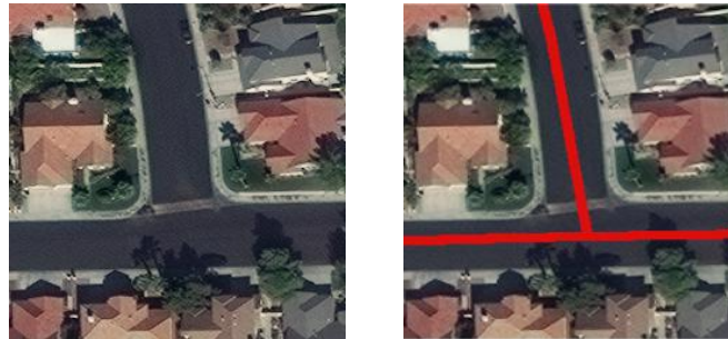
Figure 3.7: Constant two meter wide Road Detection Learning task. From Left to Right: satellite image, corresponding ground truth mask
