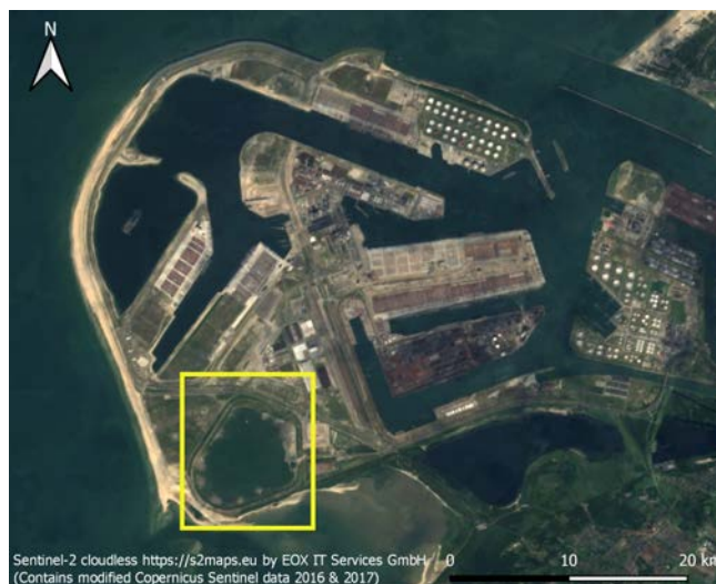
Figure 2.21: The Slufter storage basin for polluted sediment (yellow box) ( Sentinel-2 cloudless 2020 by EOX IT Services GmbH is licenced under CC BY-NC-SA 4.0).
