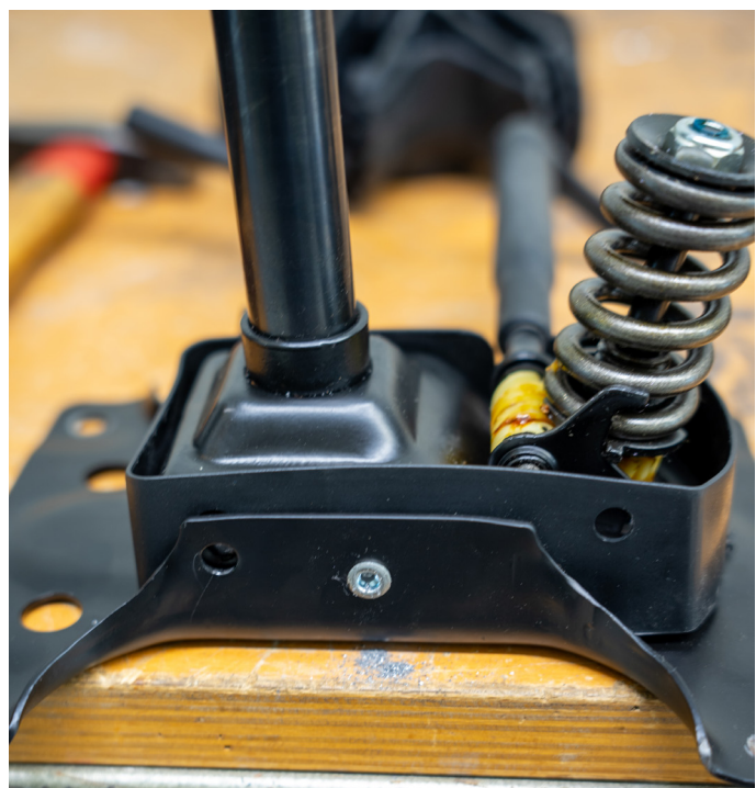
Figure 5.4 . Components of the task chair mechanism, showing (a) lubricated parts prior to disassembly, and (b) the underside of the chair, illustrating the complexity of the assembly and the difficulty of disassembly.
