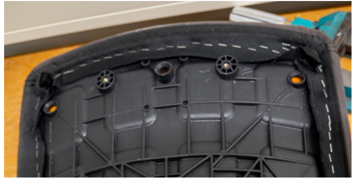
Figure 5.3 . Textile stapling practices observed during disassembly, showing (a) mesh stapled directly onto the structural seat pan, and (b) mesh stapled onto the nylon backrest structure
