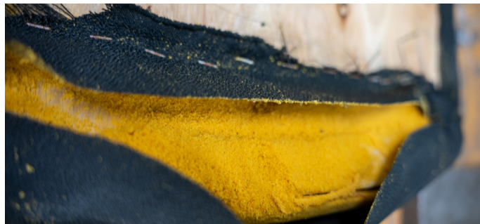
Figure 5.3 . Textile stapling practices observed during disassembly, showing (a) mesh stapled directly onto the structural seat pan, and (b) mesh stapled onto the nylon backrest structure
