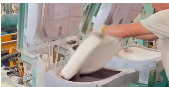
Figure 5.7. Manufacturing process of polyurethane foam, showing (a) injection of the foam mixture into the mould, (b) closing of the mould during expansion and curing, and (c) removal of the cured foam by a worker without respiratory protective equipment.
