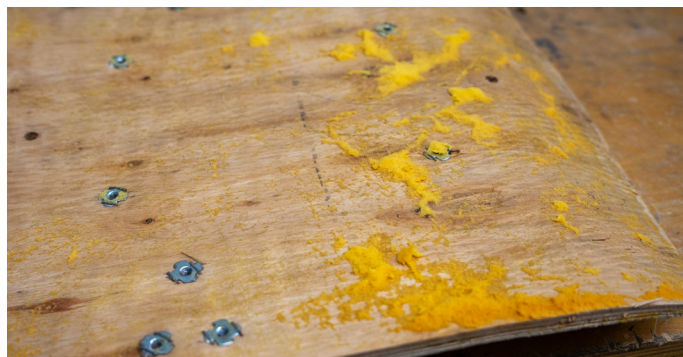
Figure 5.2 . Foam attachment methods observed during disassembly, showing (a) stapled foam attachment in the second chair, and (b) adhesive-bonded foam embedded in the structural seat pan of the first chair.
