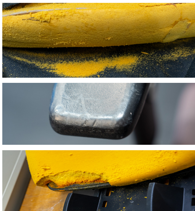
Figure 5.1 . Degradation of foam components in the disassembled task chair, showing (a) worn and chipped TPU armrest pad, (b) brittle and discoloured seat foam with visible particulate matter, and (c) detached foam fragment from the seat cushion.
