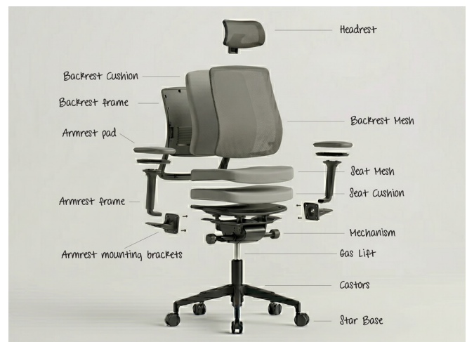
Figure 3.1 Exploded view of a typical office task chair, showing its main components.
