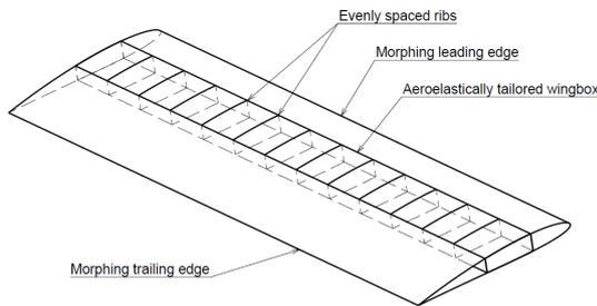
**Figure 2.** Initial structural layout of the wing.
