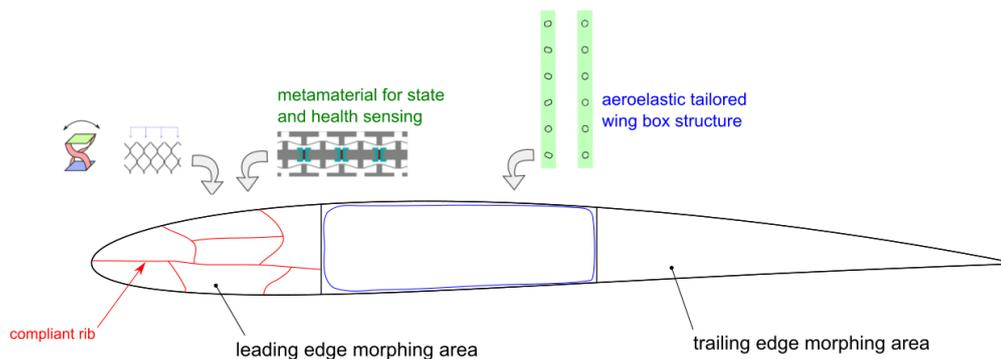
**Figure 1.** Wing section illustrating the morphing wing concept.
