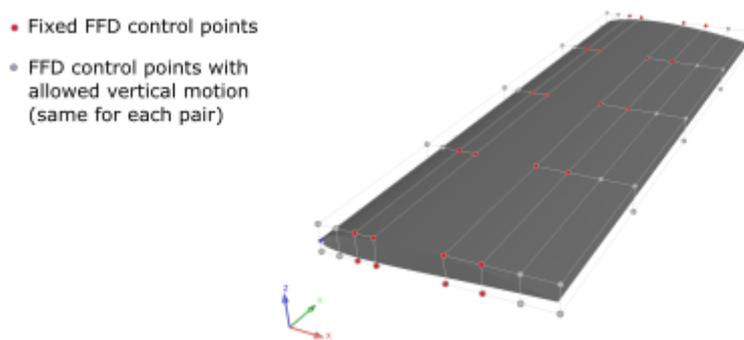
**Figure 6.** Lattice of control points of the Free-Form Deformation parameterisation.
