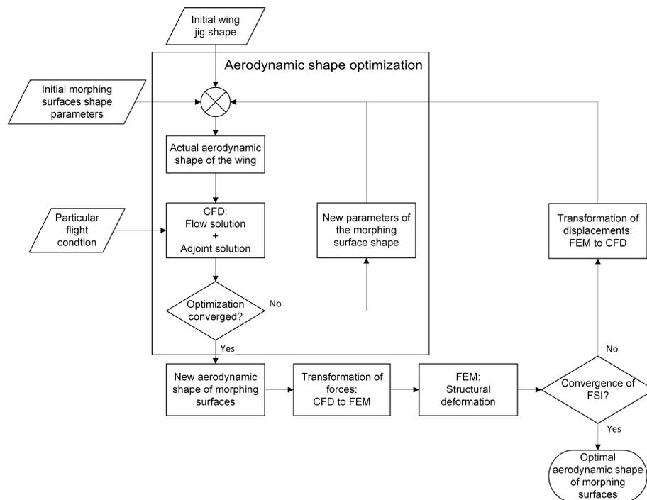
**Figure 4.** Schematics of the process for the morphing shapes aerodynamic design.
