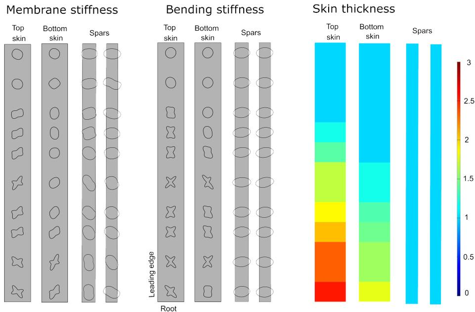
**Figure 8.** Thickness and relative directional stiffness of tailored parts of the optimised wingbox.
