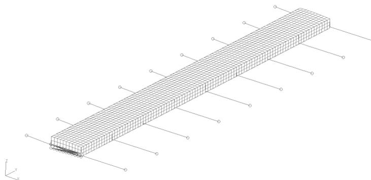
**Figure 7.** Finite element model of the wingbox for Nastran solver.
