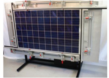
fig. 4.4.1: BrightSpot Automation mechanical testing tool (source: bibliography 4.2)
