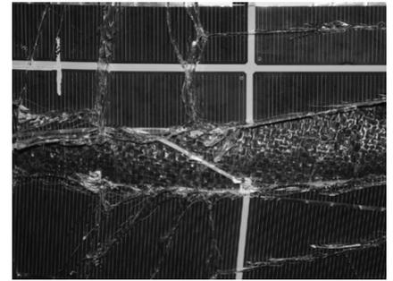
fig. 4.4.4: Improved residual resistance due to PV wafer cells' soldered inter-connectors
