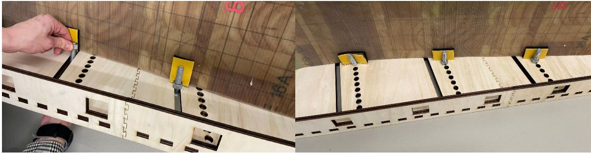
Figure 78: Slotted bolt (left) and perforated bolts in the connection points along the height of the cassette. Rubbers are placed between the bolt / nut combination and the panel.
