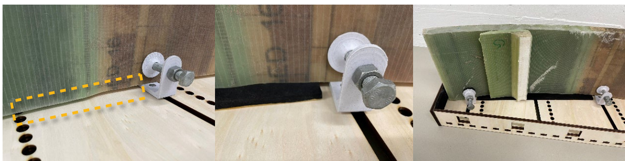
Figure 86: A) The clamp creates a +5 mm gap between the panel edge and backplate of the cassette. B) allowing for good acoustic sealing, C) without the problem of inconsistent panel thickness.
