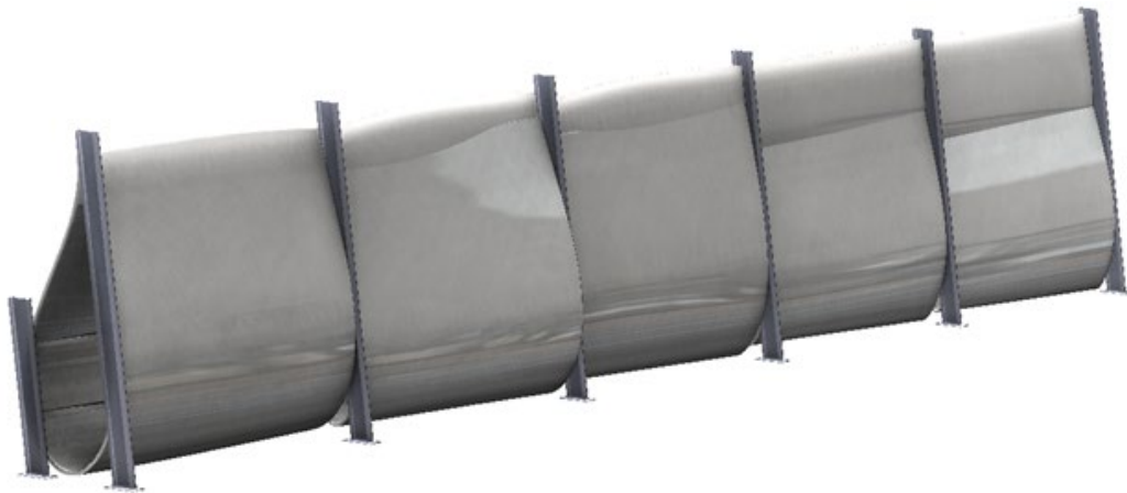
Figure 41: Segments concept with tilted, opposing T- or IPE-frames. The irregularities in all sections but the leftmost one come from stacking of segments which was needed to reach a common height.
