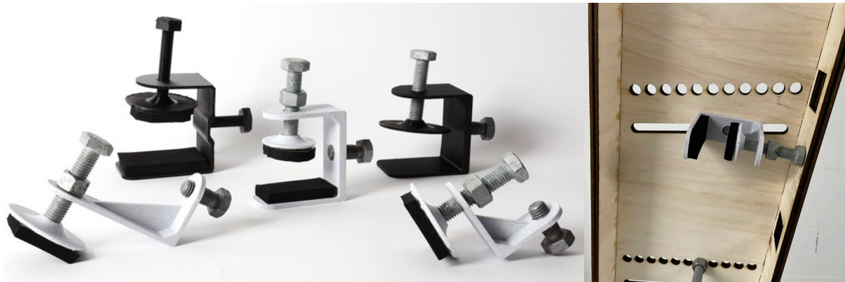
Figure 79: A) Adjustable clamp designs, multiple iterations. Improvements mainly covered better 3D printability (thinner flanges), stiffness (larger thickness, ribs) and fitting of steel M12 bolts. B) tested clamp.
