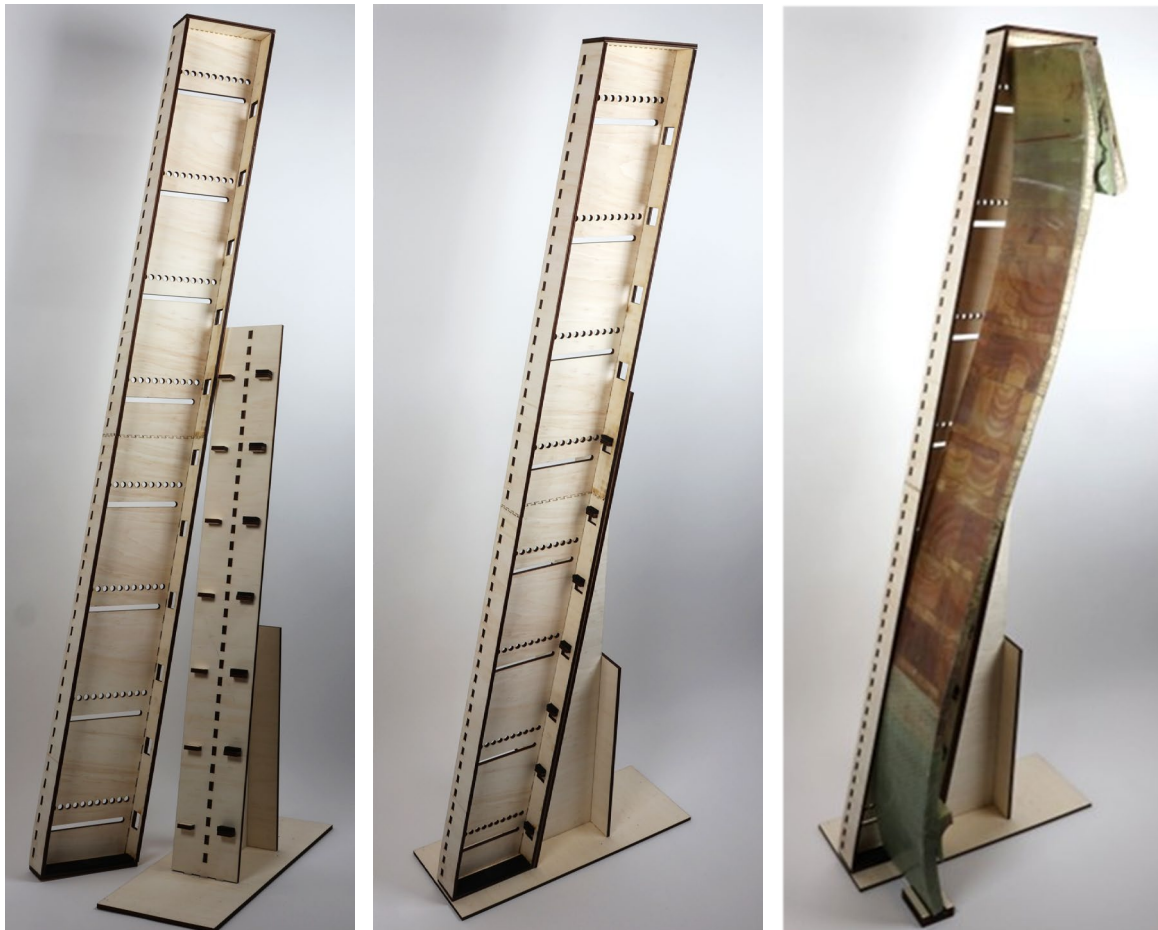
Figure 77: A) the wooden cassette with perforations and slots in the backplate and the mounting structure on the frame part. B) the three parts assembled into the demonstrator prototype.
