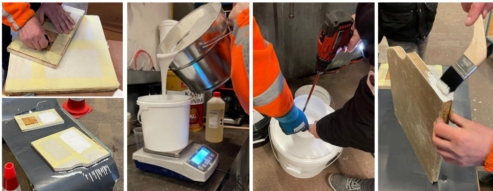
Figure 87: Taping and sanding the panels, mixing the epoxy coatings, applying them on cutting edges and front surfaces, and letting them dry for the pull-test.
