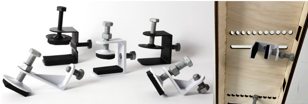
Figure 124: A) Adjustable clamp designs, multiple iterations. Improvements mainly covered better 3D printability (thinner flanges), stiffness (larger thickness, ribs) and fitting of steel M12 bolts. B) tested clamp.
