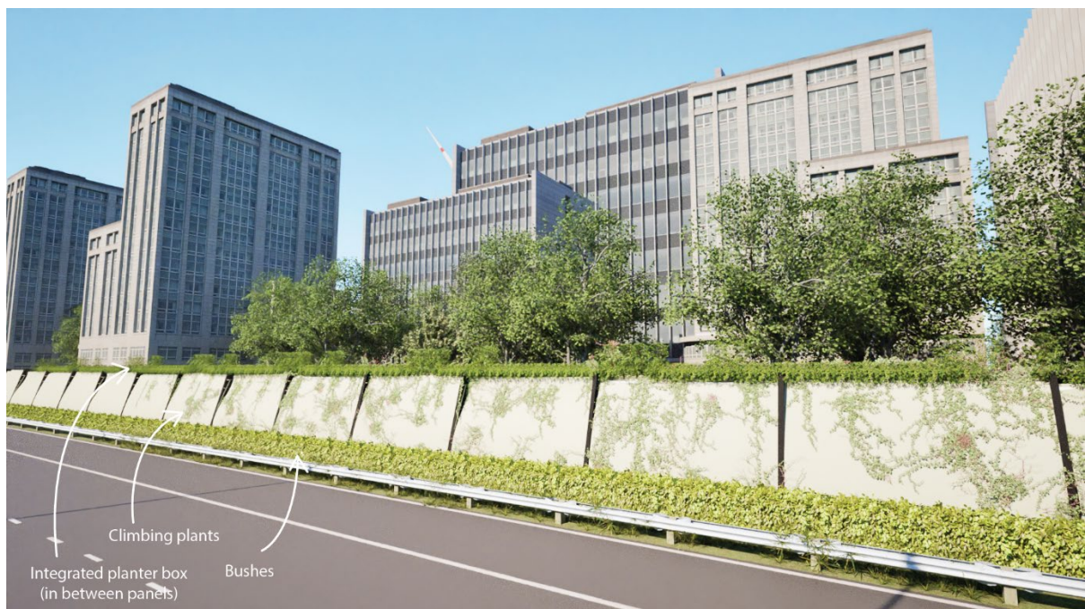
Figure 93: The noise barrier design in an urban environment, with three vegetation options: climbing plants, integrated planter box and vegetation around the barrier. This can also work on the resident side.
