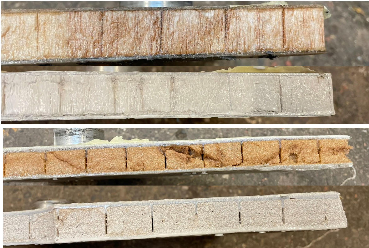
Figure 88: 24 hours after coatings were applied to cutting edges. The coatings seems to be smoother and less absorbed by the balsa wood (top), as compared to the foam core (bottom). The white EP510 coating seems to be less absorbed by both panels. This might be due to its higher viscosity.
