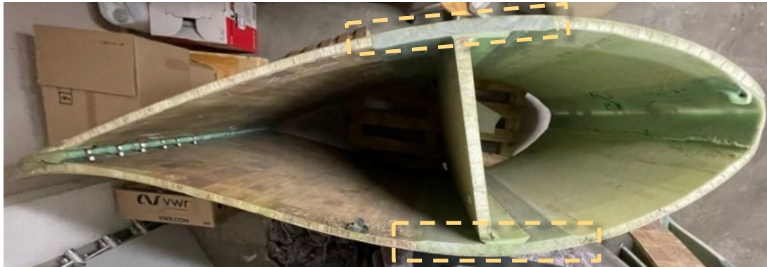
Figure 13: Photo of a WTB segment. The LE panels and shear web are made of GFRP-foam sandwich, while the TE panels are GFRP-balsa. The spar cap (boxed) is a complete block of GFRP.
