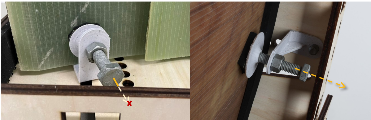
Figure 84: By making longer clamp flanges (as done in right image), extending clamp bolts will move over the cassette side instead of colliding into it.
