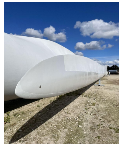
Figure 9: Almost flat tip of a 45 m long Vestas V90 blade on a field.
