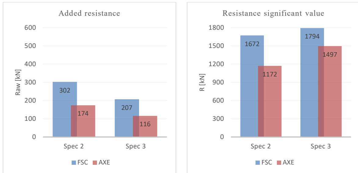
Figure 18: Comparison of the resistance of the FSC and AXE frigate at 26 knots
