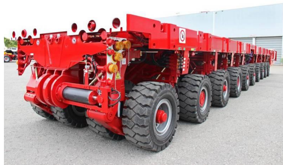
Figure 10.4: Self Propelled Modular Transporter (SPMT) [54]
