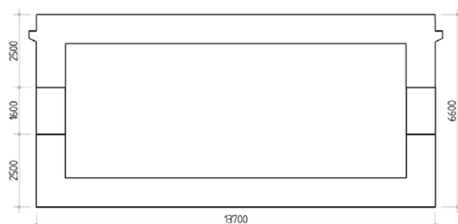
Figure 8: Cross-section underpass - Layout H
