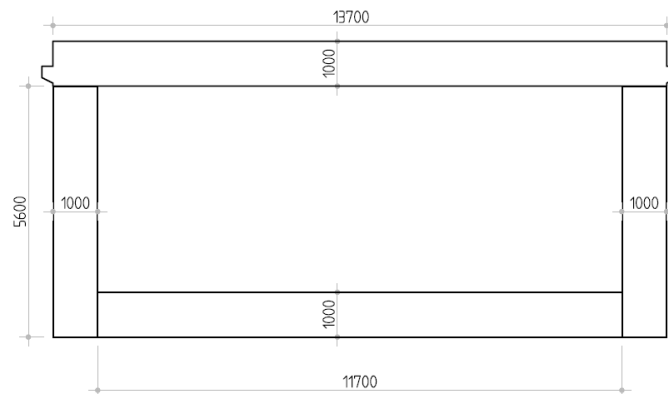
Figure 6.4: Cross-section underpass - Layout D
