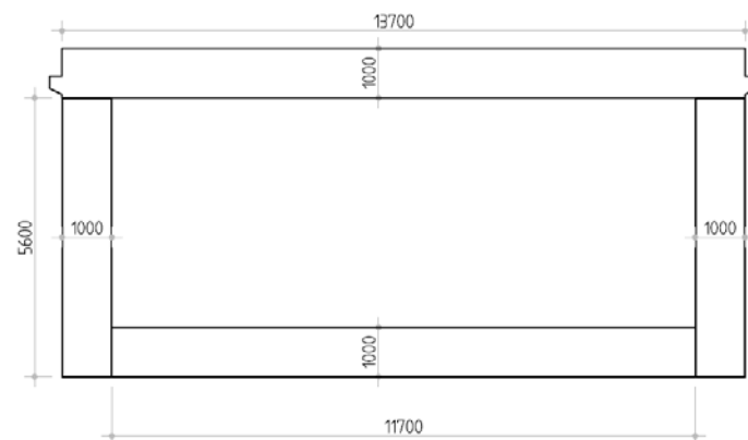
Figure 4: Cross-section underpass - Layout D
