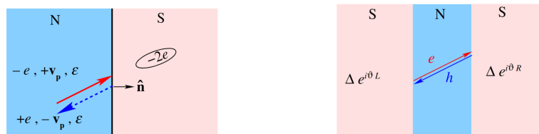
Figure 2.7: Left. An illustration of Andreev reflection at a normal-superconductor (N-S) interface. The charge, velocity and energy of the electron and hole are labeled. Right. Schematic for an Andreev bound state through repeated AR in an S-N-S junction. The superconductors have a phase difference \phi = \theta_L - \theta_R . Drawings adapted from [41]
