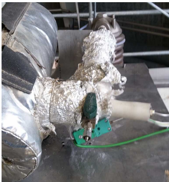
Figure A4.4. Point of SPA sampling; location downstream the reactor
