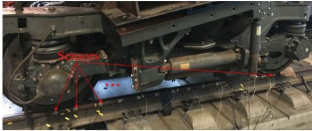
**Figure 9.** The tested bogie-track system in laboratory and the acceleration sensors.
