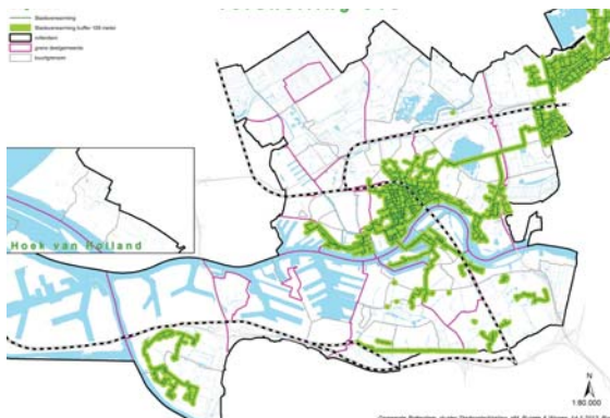
current district heating pipelines
