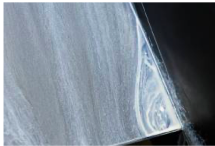
Figure 2.4: Oil-flow visualizations in the trailing-edge corner of the F6 wing from Kegerise et al. [20]
