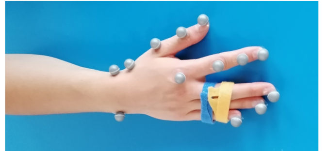
Figure 3: Marker configuration used with the motion capture system to record the pinch tasks. Markers at the EM and EL landmarks are not visible in the image, but were present during the recordings.
