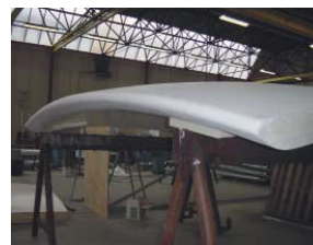
FIG. 143 Fourth prototype, a prefab sandwich construction
