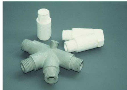
FIG. 212 Polystyrene moulds with an aluminium node
