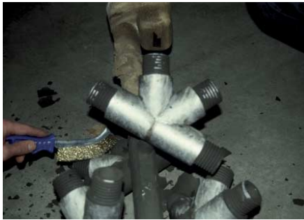
FIG. 209 Space frame node
