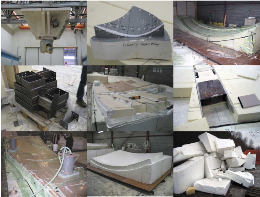
FIG. 147 Milling machine at Marin, scale model of upper wing of 'The Library' and production of the roof segments at Holland Composites. Vacuum injection of the top layer on foam block milled by Marin. Insert to be placed in the GRP sandwich roofs in order to make a connection between the roofs and the columns [34 & 36]. Placement of foam blocks and glass fibre mats, which will become stringers. Vacuum injection of the bottom layer. Final result, in this case an early prototype. Discarded foam moulds
