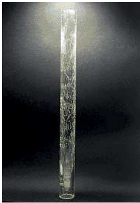
FIG. 86 Laminated glass column
