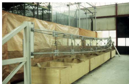
FIG. 73 Mock-up scale 1:2 in Octatube Laboratory just before abortion of the experimentation process
