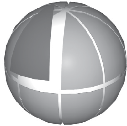
FIG. 128 Scheme of the proposed division: 2 x 8 spherical segments in GRP
