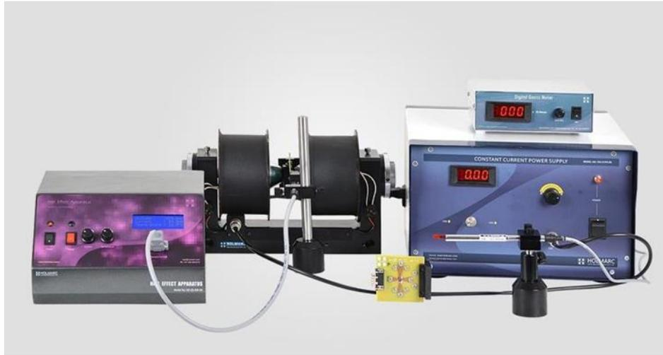
Figure 58 Hall measurement setup [105]
