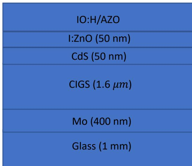
Figure 48 CIGS solar cell architecture
