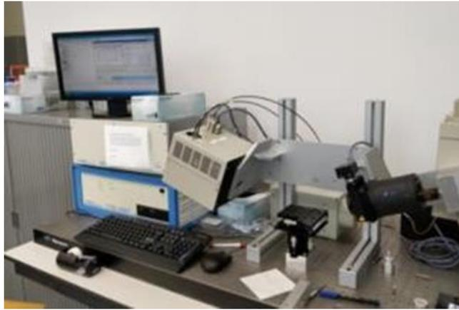
Figure 55 Ellipsometer setup
