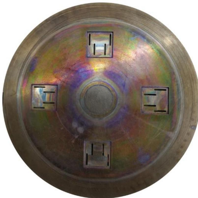
*Figure 47 Sample holder used to perform deposition of IO:H on CIGS solar cells*
