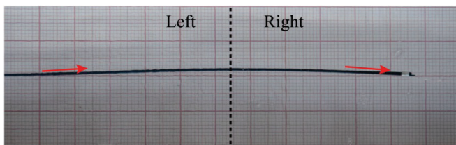
Figure 3.10. Final position of the needle inside the gelatine during the trial in which the steering direction was changed from left to right ( BO = 0.9 mm, S = 2.0 mm). Arrows showing the direction of steering and the middle-dashed line point when direction changed.
